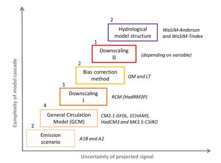
Figure 2 The model cascade is depicted with the individual members of each component listed on the right. Permuting the members of all components (Downscaling I and II are only shown for the sake of completeness) results in a total of 32 hydrological projections.
