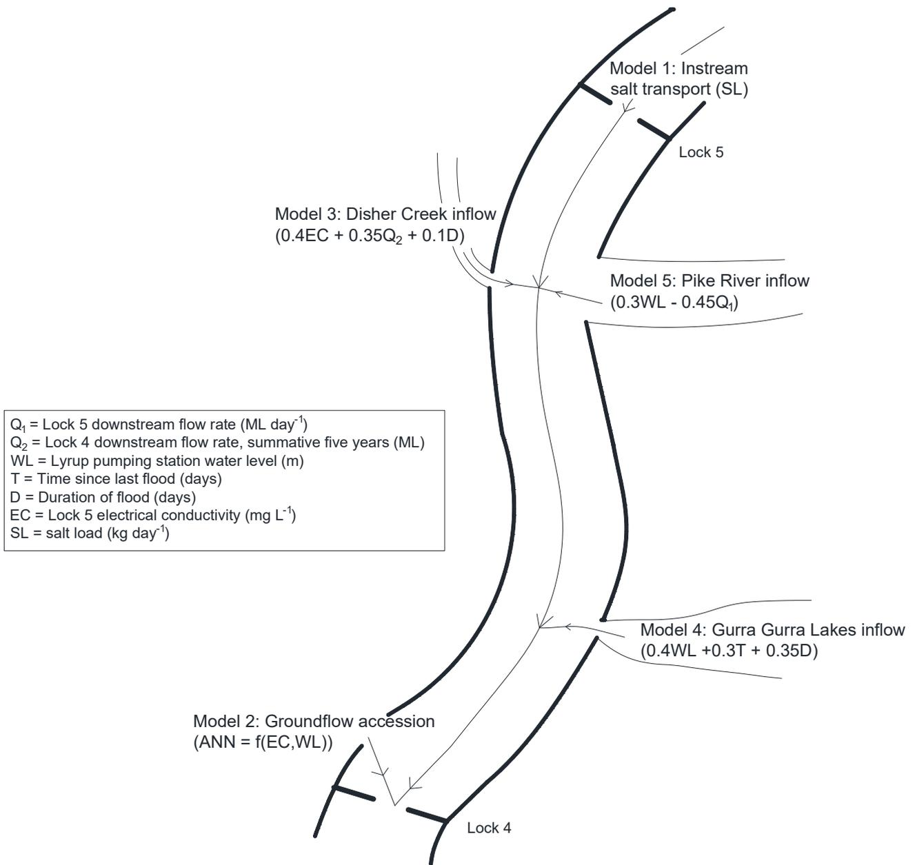
545 **Figure 7. Schematic of the hybrid model on a stylised view of the river (not to scale). The regression models are input as point loads, while the groundwater accession is added to the transport model at Lock 4.**
