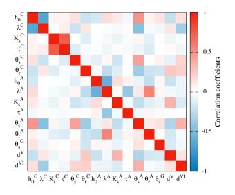
**Figure 11.** The correlation coefficients for the mean parameter set show in particular that the porosity of the gravel layer ( $\theta_s^G$ ) as well as the position of the material layers ( $d^V$  and  $d^{VI}$ ) can be reliably estimated from single-channel GPR when evaluating both the signal travel time and amplitude.
