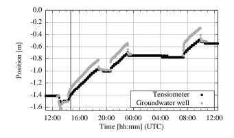
**Figure 2.** During the experiment with two distinct phases (initial drainage and multistep imbibition – separated by the vertical line), the position of the groundwater table was measured manually in the groundwater well and automatically with the tensiometer (Fig. 1). The difference between them is proportional to the driving force of water flow in the gravel layer.
