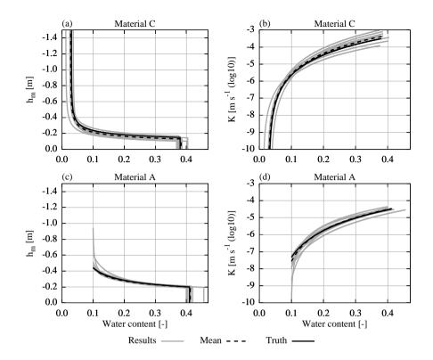
**Figure 10.** The resulting material parameters estimated from synthetic data are shown for the 10 best ensemble members (Sect. 3.1.2) together with the mean of these parameter sets and the true parameter set (Table 2). The plot range of the parameters is adjusted to the water content range of the data.
