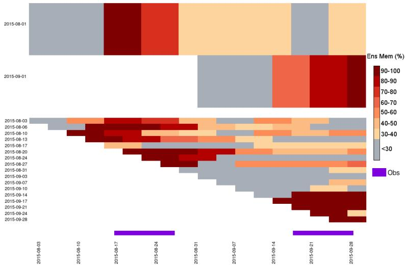
**Figure 4.** Percentage of ensemble members predicting low flow anomaly (< 97%) on the Rhine river north of Cologne for summer 2003. The two starting dates in August and September from SYS4 are compared to the 17 starting dates of the seamless forecasting system. In two separate events the discharge was recorded below the 97 % percentile, event 1 on 17-27 of August and event 2 on 18-28 of September 2003.
