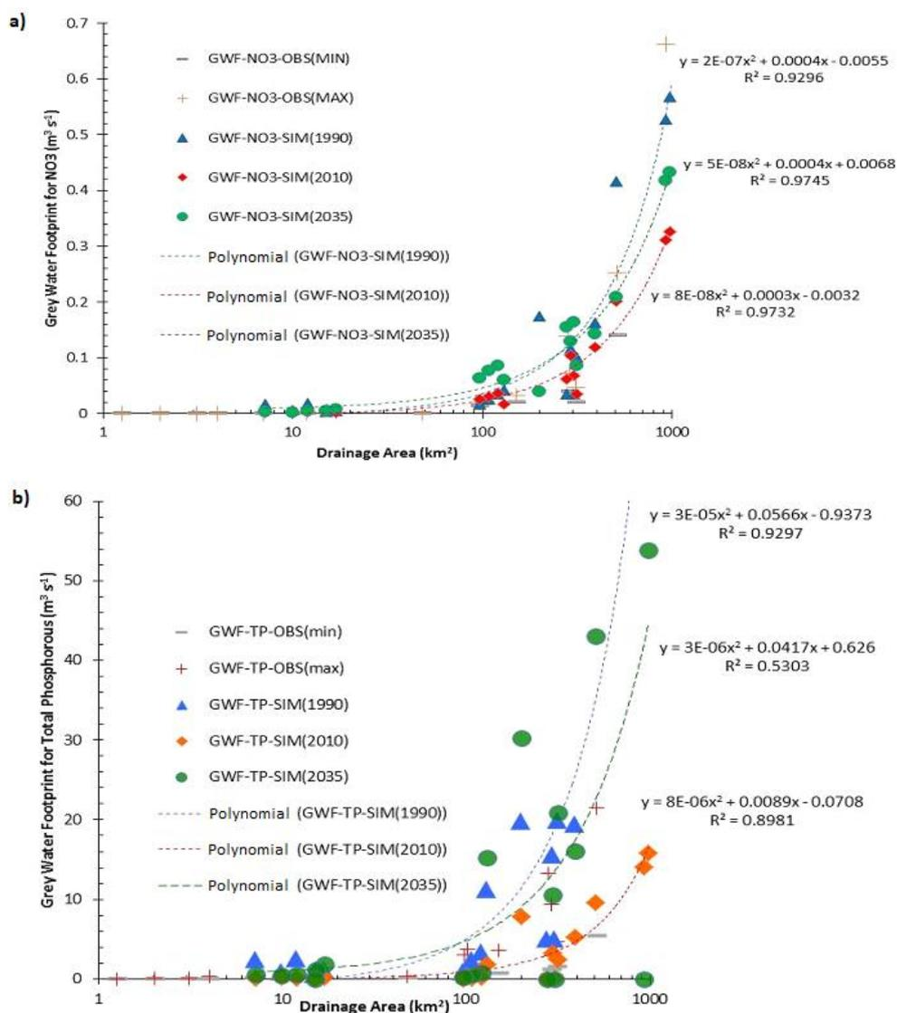
**Figure 15:** Relationships between Grey Water Footprint for Nitrate (a) and Total Phosphorous (b) according to three LULC scenarios (1990, 2010 and 2035) and size of the drainage areas of headwaters in the Cantareira Water Supply System.
