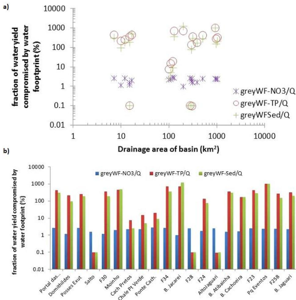
**Figure 12:** Fraction of water yield compromised by the grey water footprint for nitrate, total phosphorous and sediments versus drainage area (a), and showing the studied subbasins (b).
