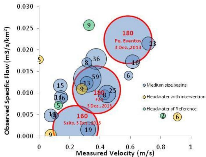
**Figure 6:** Experimental sampling of turbidity (size of circles), observed flows and mean velocities in river cross sections of 17 catchments in Cantareira System headwater (Oct, 2013 - May, 2014).
