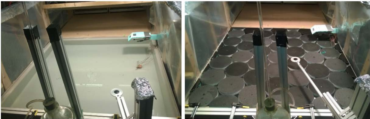
Figure A: The water basin with 1.2×1.2 m 2 surface area and 0.16 m depth at the end of a wind tunnel built in our laboratory (STEP - ETH Zurich); uncovered basin (left) and covered with black discs (right). The experiments were conducted for a series of boundary conditions with black and white covers (not shown here).
