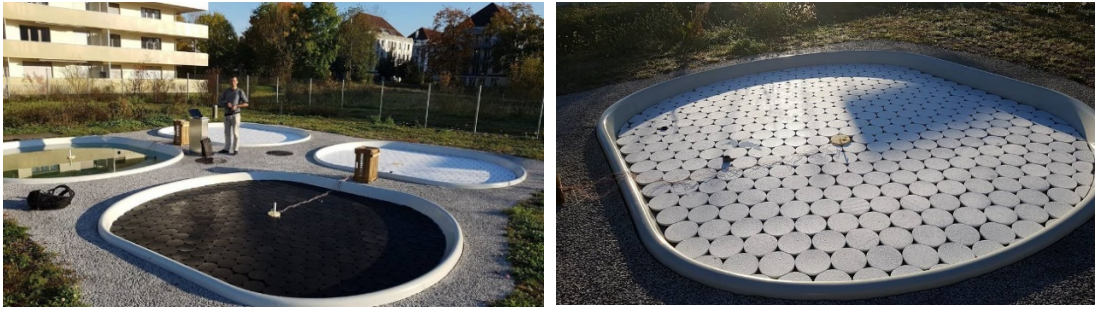
Figure C. Ongoing “field scale” experiments conducted in EAWAG near Zurich using 8 ponds each 14 m 2 and 1.5 m deep covered with white and black 0.2 m (EVA foam) floating covers including two uncovered control ponds
