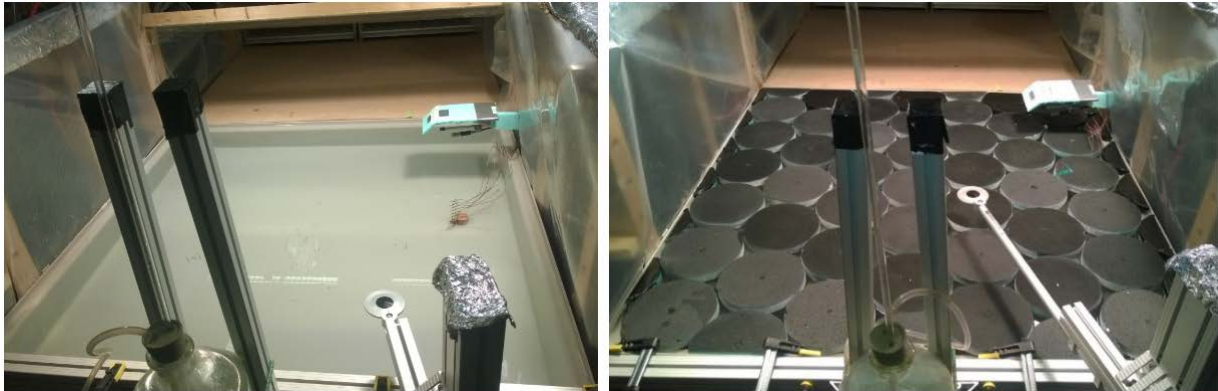
Figure A: The water basin with 1.2 \times 1.2 \text{ m}^2 surface area and 0.16 m depth in our laboratory; uncovered (left) and covered with black discs (right)
