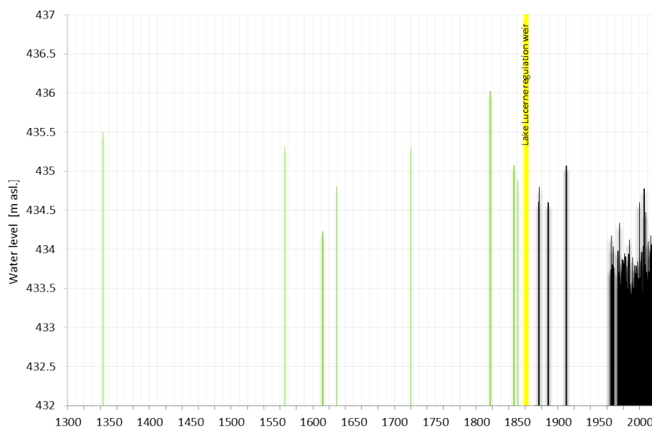
9 Figure 12: Long term stationarity of Lake Lucerne and Reuss River extreme flood water levels (Wetter 10 et al., 2015b) or slow trend of decreasing flood magnitudes (?) 11 Green bars: reconstructed flood levels above sea level (asl.) 12 Black bars: measured flood levels asl. 13 Yellow bar: significant anthropogenic intervention in the discharge conditions
