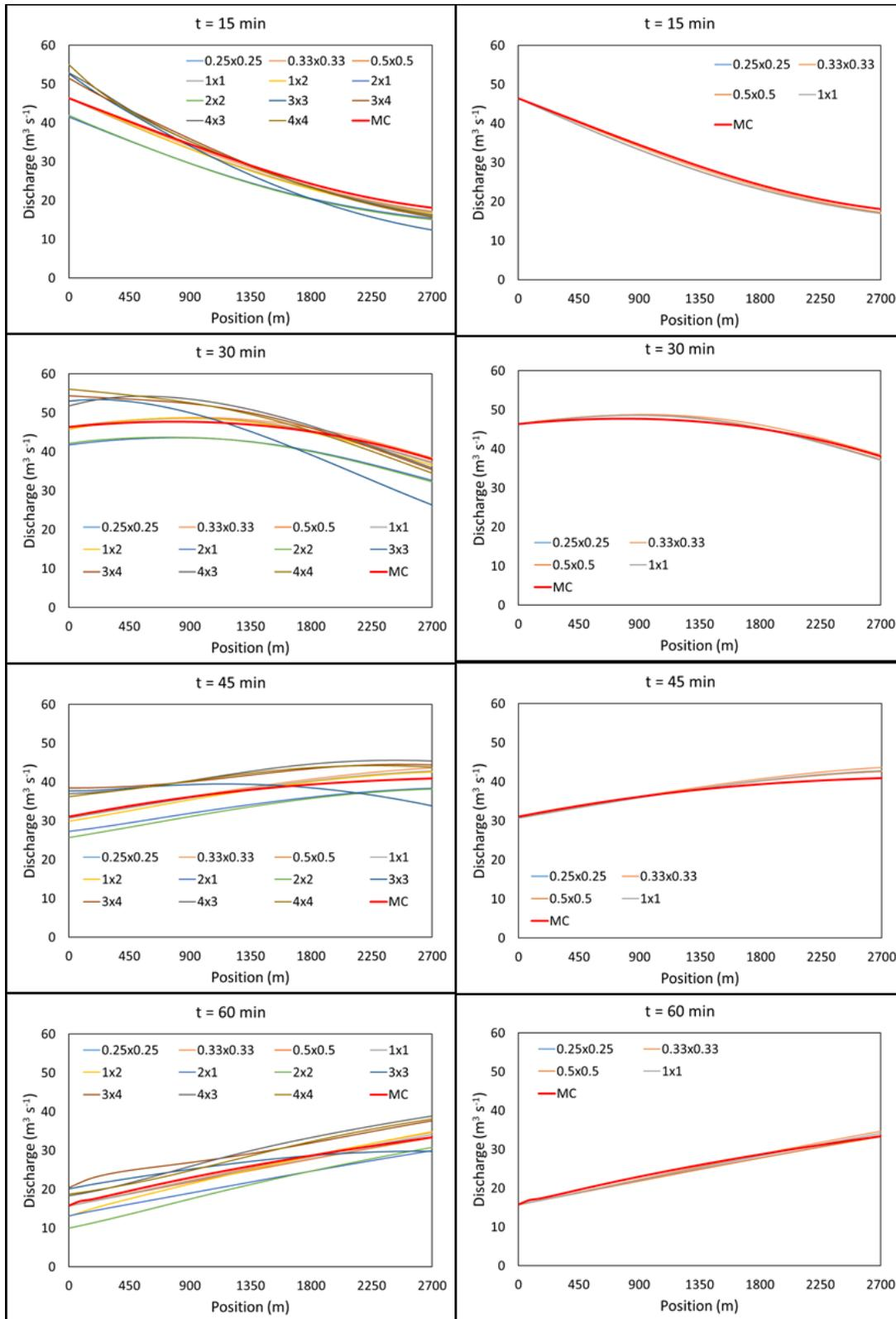
Figure 4. Plots of discharge results obtained from the FPE methodology solved using different  $\alpha$ - $\beta$  discretizations. The results of the Monte Carlo (MC) simulations are also plotted for comparison (thick red line). The figures on the left show all the different discretizations attempted; the figures on the right show only the few discretizations closest to the one used in the manuscript (0.5x0.5).
