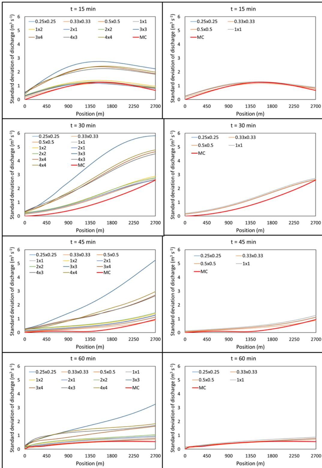
Figure 5. Plots of the standard deviation of discharge results obtained from the FPE methodology solved using different  $\alpha$ - $\beta$  discretizations. The results of the Monte Carlo (MC) simulations are also plotted for comparison (thick red line). The figures on the left show all the different discretizations attempted; the figures on the right show only the few discretizations closest to the one used in the manuscript (0.5x0.5).
