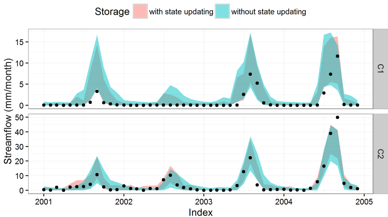
5 Figure 5 Representative time series of the 90th percentile prediction limits, with observed values as black dots, for the 10 year calibration period observed rainfall models. State updating can be seen to increase precision compared to without state updating.
