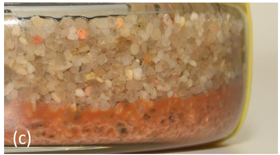
Figure S5: Distributions of (a) NMR porosity and (b) mean relaxation times of sample F4 after precipitation of ferrihydrite (c).
