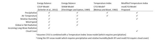
Fig. 1. Required forcing data for the COUP, SHAW, CFGI, and modCFGI frozen ground models.
