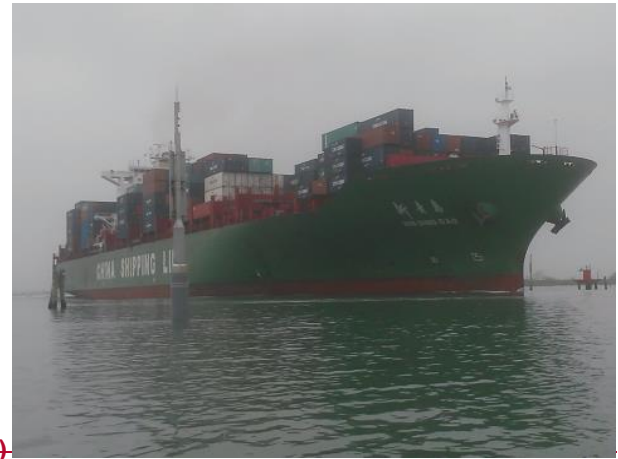
Figure 4: (a) Water level (m above msl) recorded on the bottom of the MMIC and computed by SHYFEM on the tidal flat 300 m far from the channel caused by the transit on April 6, 2016, of the Cargo-Hazard A. A photo of the vessel is shown in (b). The commercial vessel, which was used as reference, is 280 m long, 40 m wide, and characterized by a gross tonnage of 66433 t. The ship speed s was equal to 8.1 knots (4.2 m/s). The time steps T1-T6 highlighted by red dots in (a) refer to the model outcome shown in Fig. 10.
