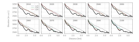
**Figure 12.** Bedrock topography (thick black lines) and simulated glacier thickness (thin colored lines) along the centerline of Hintereisferner as simulated for a single GCM-RCM combination (REMO2009 driven by MPI-ESM-LR) and the three RCPs, shown in 10-year intervals. Dashed black lines indicate the initial ice thickness as of the year 1997.
