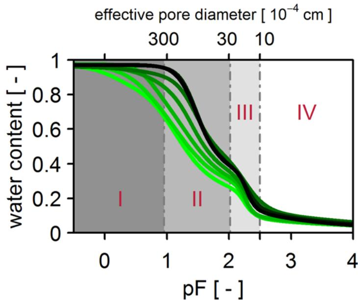
5 Figure 8: Four pore domains represented in the soil water retention curve. The roman letters I-III denote different capillary water domains for which a detailed explanation is given in the text and values are presented in Table 4. The region denoted by IV is non-capillary (residual) water.
