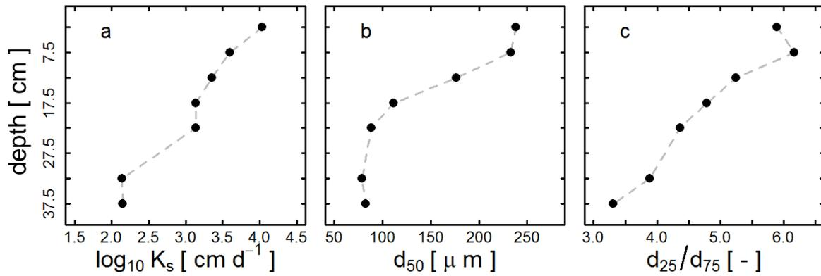
Figure 7: (a) Trends of key pore systems characteristics with depth: (a) near exponential decrease in  $K_s$  with depth, (b) decrease of characteristic pore diameter with depth, expressed as median pore diameter  $d_{50}$  of the second modality (c) reduction of the width of the pores-size distribution with depth, expressed by  $d_{75}/d_{25}$ .
