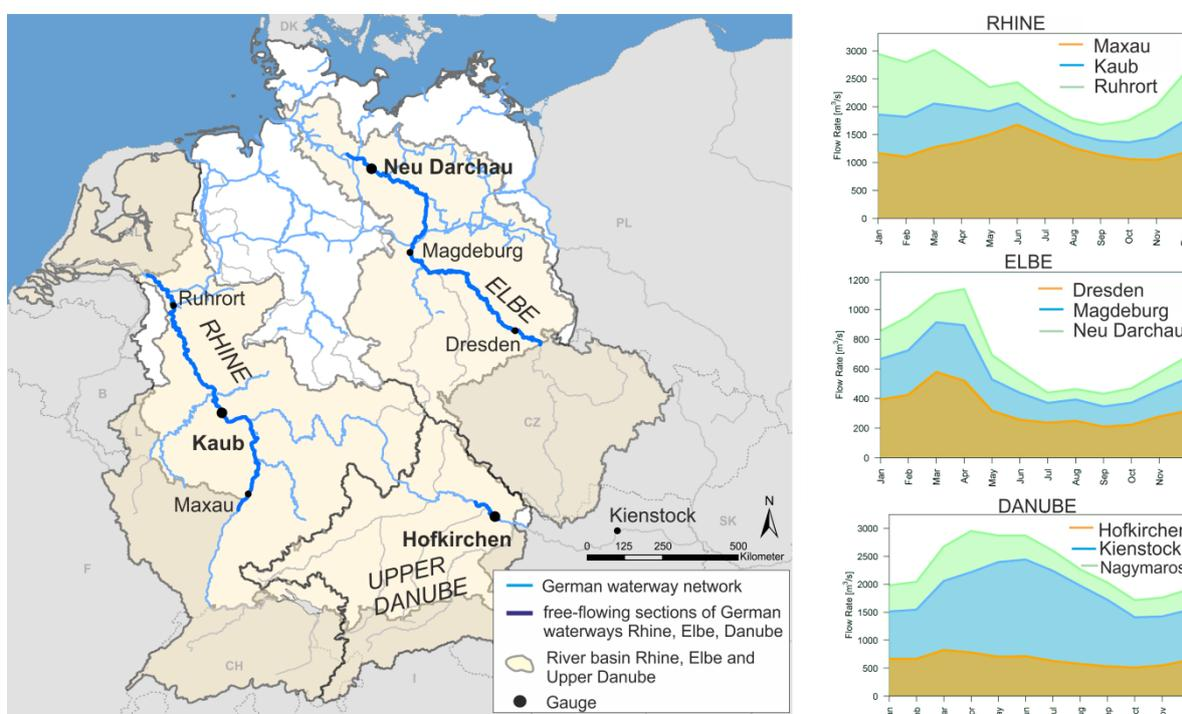
**Figure 2.** Map showing the German stretches of the international waterways Rhine, Danube and Elbe (left part), for relevant gauges (black dots) the long-term monthly mean flow rates (1981-2000) are visualized (right part).
