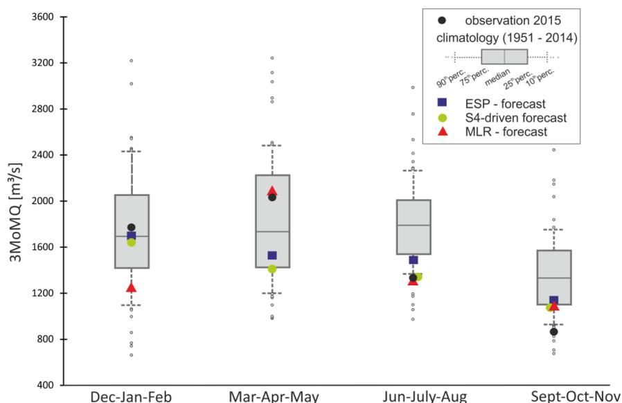
**Figure 13.** Comparison between the three navigation-related forecast approaches for the monthly mean flow of the next three months 3MoMQ initialized in December 2014, March 2015, June 2015, September 2015 (meteorological seasons 2015) at gauge Kaub /Rhine in relation to the observed values and the climatology (1951 – 2014).
