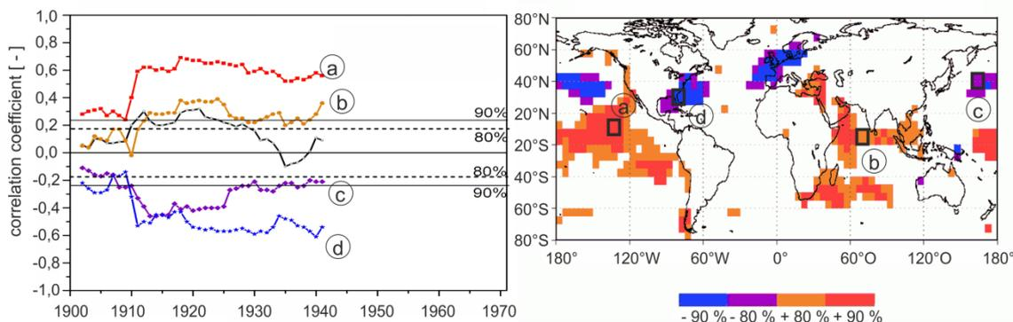
**Figure 4.** Example of a stability correlation map. Left: correlation between streamflow and SST of a 31-year moving window for selected grid areas; right: map showing the areas with stable positive or negative correlations.
