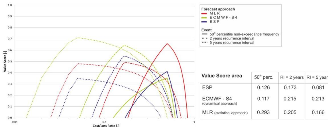
10 **Figure 9.** Economic value score plotted against cost-loss ratio for three forecast approaches predicting the lowest seven day mean MoNM<sub>7</sub>Q of the next month at the gauge Kaub / Rhine for three different event thresholds within the typical low flow season July to November (verification period 1981 – 2014).
