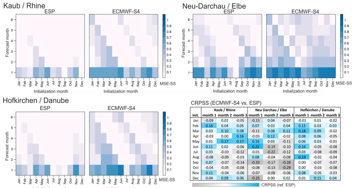
5 **Figure 6.** MSE-SS for ESP and S4-driven forecast for each initialisation and forecast month at the stations Kaub, Neu Darchau, Hofkirchen and CRPSS values of S4-driven forecast related to ESP for forecast month 1 to 3 (verification period 1981 – 2014).
