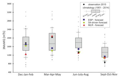
**Figure 13.** Comparison between the three navigation-related forecast approaches for the monthly mean flow of the next three months 3MoMQ initialized in December 2014, March 2015, June 2015, September 2015 (meteorological seasons 2015) at gauge Kaub /Rhine in relation to the observed values and the climatology (1951 – 2014).
