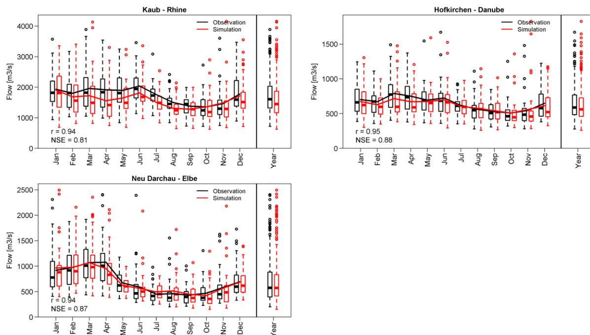
**Figure 3.** Comparison of the simulated (red) and observed (black) long-term (1981-2015) monthly mean streamflow and the distribution of the simulated and observed monthly mean streamflow within the different months and for the whole year illustrated as box-plots of the gauges Kaub - Rhine (top left), Hofkirchen – Danube (top right) and Neu Darchau – Elbe (bottom).
