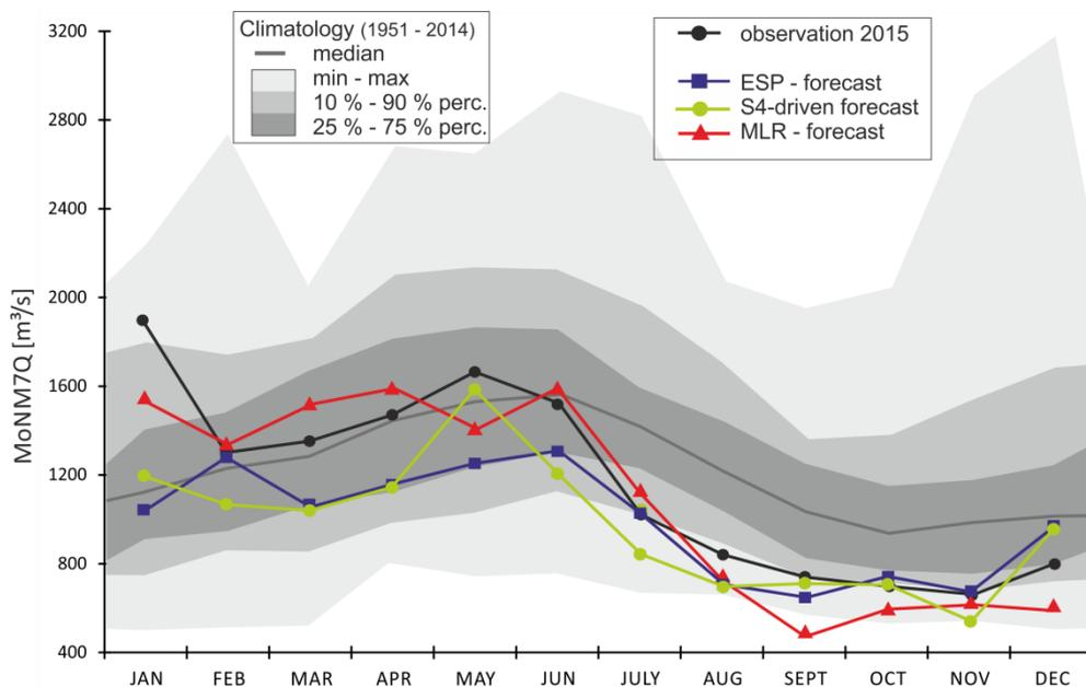
**Figure 12.** Comparison between the three navigation-related forecast approaches for the lowest seven day mean MoNM<sub>7</sub>Q of the next month in the year 2015 at gauge Kaub / Rhine in relation to the observed values and the climatology (1951 – 2014).
