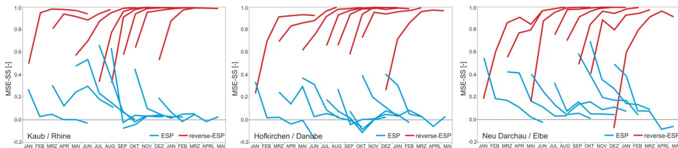
**Figure 5.** MSE-SS of the ESP (blue) and reverse ESP (red) forecast (reference: simulated to the MSE from using a climatology) for the gauges Kaub / Rhine, Hofkirchen / Danube and Neu Darchau / Elbe over a lead-time of 6 months (verification period 1981 – 2014).
