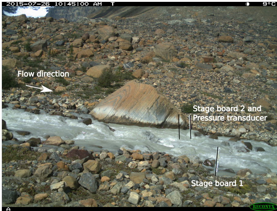
Figure 3. Reconyx raw picture showing the installation of stage boards, pressure transducer and boulder used for gauging (center of picture). Black lines represent the 3 different tested profiles.
