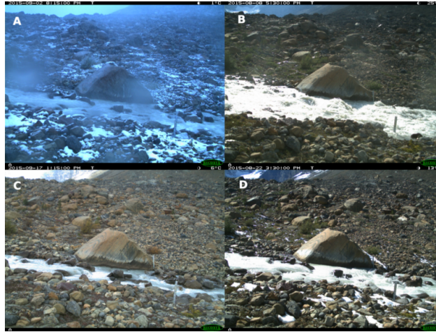
Figure 4. Images illustrating the main issues affecting image quality and measurements during the stage and width calculation: (a) heavy weather conditions (b) boulder shadow and intense water reflection (c) emerged rocks on the main channel at low flows (d) light snow cover on the edge of the stream.
