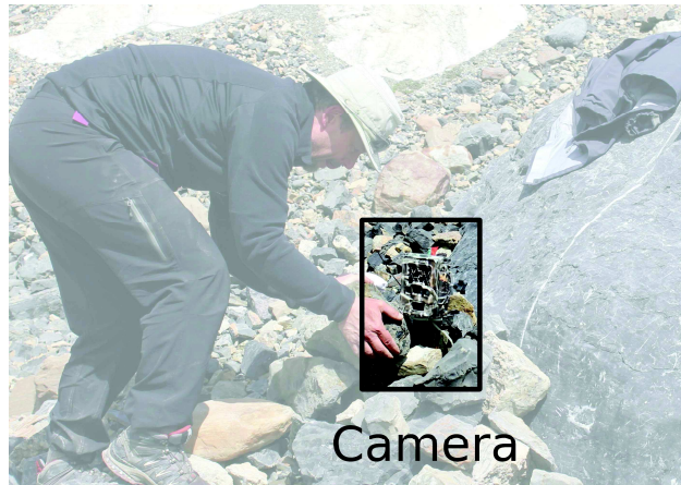
Figure 2. Camera set up. The camera is set on the right bank of the stream, a few meters above the water level. The camera is clamped to a pole hammered into the ground.
