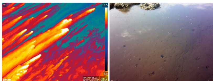
920 Figure 6: Thermal infrared (TIR) image from March 21, 2014 at Tidmarsh Farms illustrating PFP (type 2) seepage. Many macropores are observed in both the infrared (slightly smaller) and the visual image. These seeps are located in the middle of cell 3 (Fig. 1B), where peat is ~3m thick and dramatically thinning.
