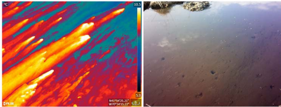
Figure 6: Thermal infrared (TIR) image from March 21, 2014 at Tidmarsh Farms illustrating PFP (type 2) seepage. Many macropores are observed in both the infrared (slightly smaller) and the visual image. These seeps are located in the middle of cell 3 (Fig. 1B), where peat is ~3m thick and dramatically thinning.
