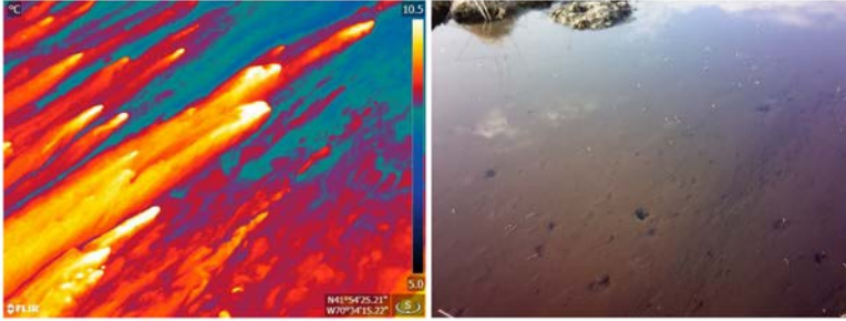
Figure 6: Thermal infrared (TIR) image from March 21, 2014 at Tidmarsh Farms illustrating PFP (type 2) seepage. Many macropores are observed in both the infrared (slightly smaller) and the visual image. These seeps are located in the middle of cell 3 (Fig. 1B), where peat is ~3m thick and dramatically thinning.
