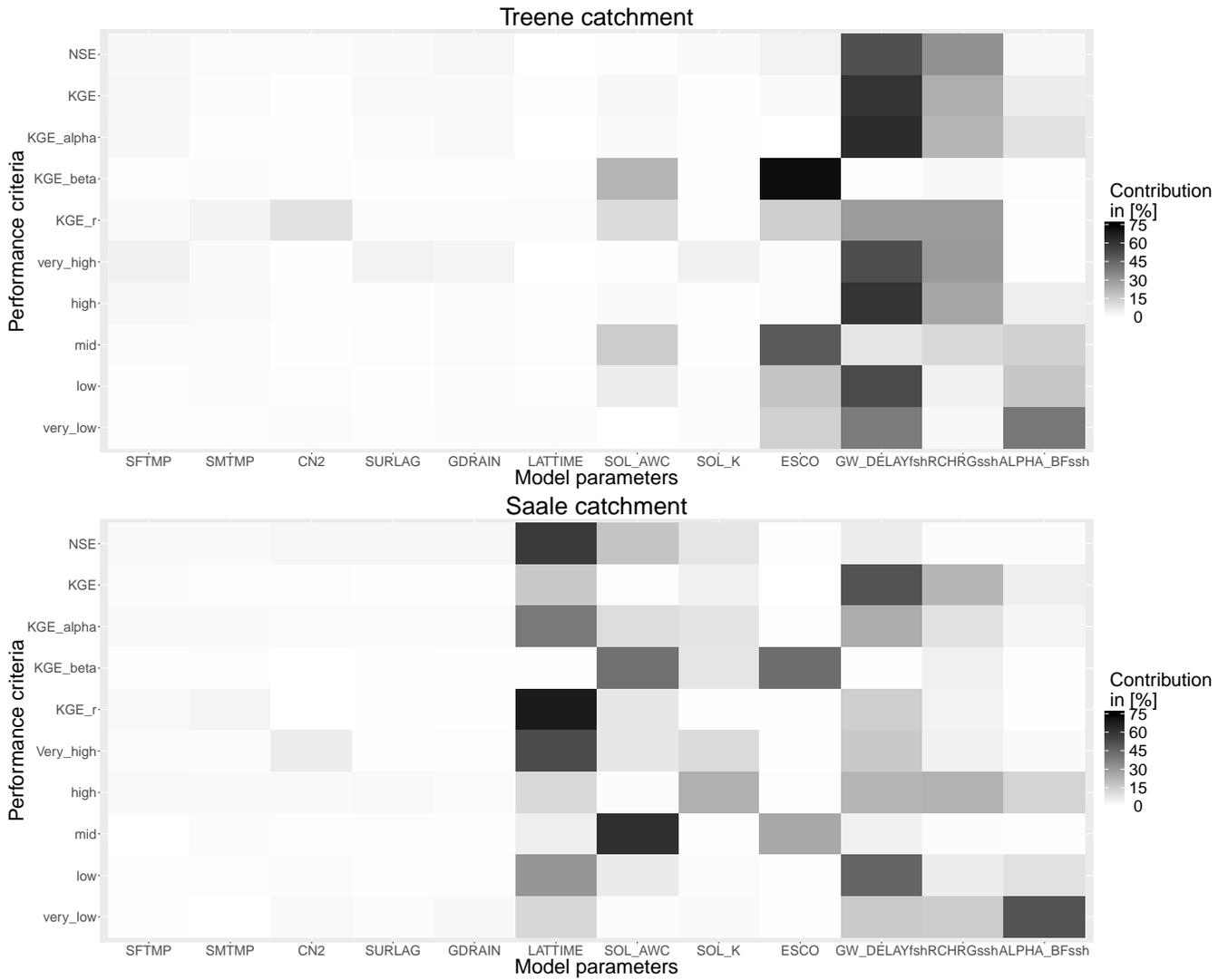
**Figure 5.** Regression trees (RT) using performance criteria as target variables. The percentage contribution of model parameters in explaining performance criteria is shown for Treene (above) and Saale (below) catchment. In every row the percentage contributions sum up to 100%.
