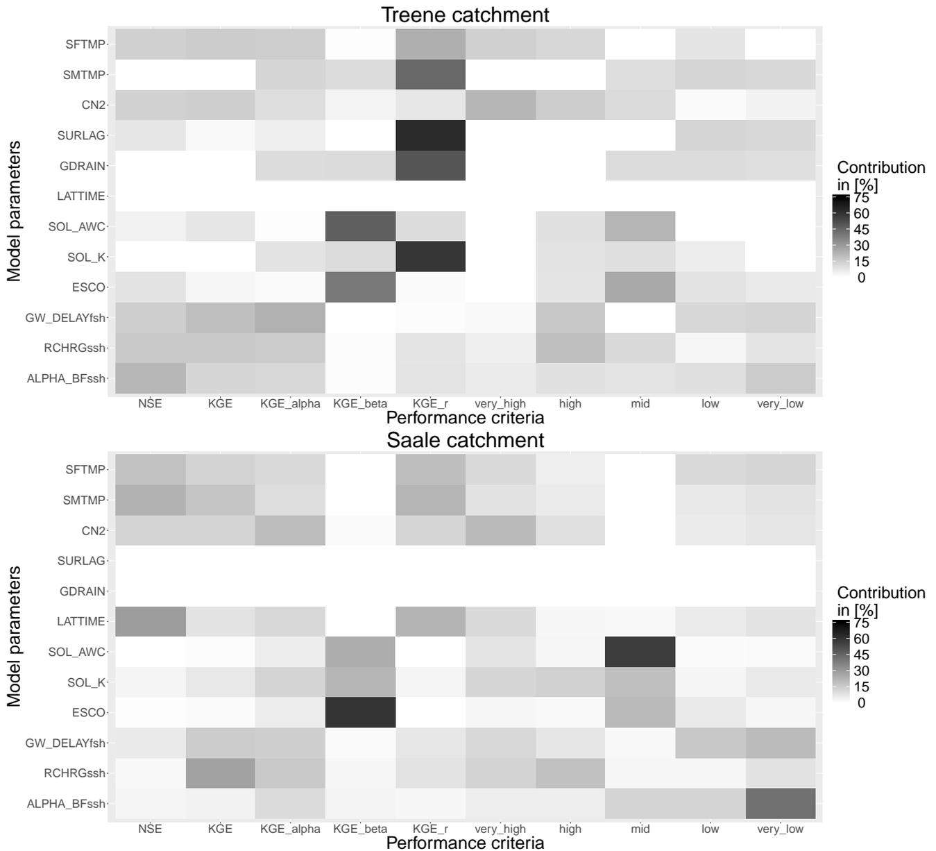
**Figure 6.** Regression trees (RT) using model parameters as target variables (RTpar) for Treene (above) and Saale (below) catchment and performance criteria as explaining variables. All values of a parameter are in white in the case that the resulting variation among performance criteria for this parameter was too low to construct a regression tree. In every row the percentage contributions sum up to 100%.
