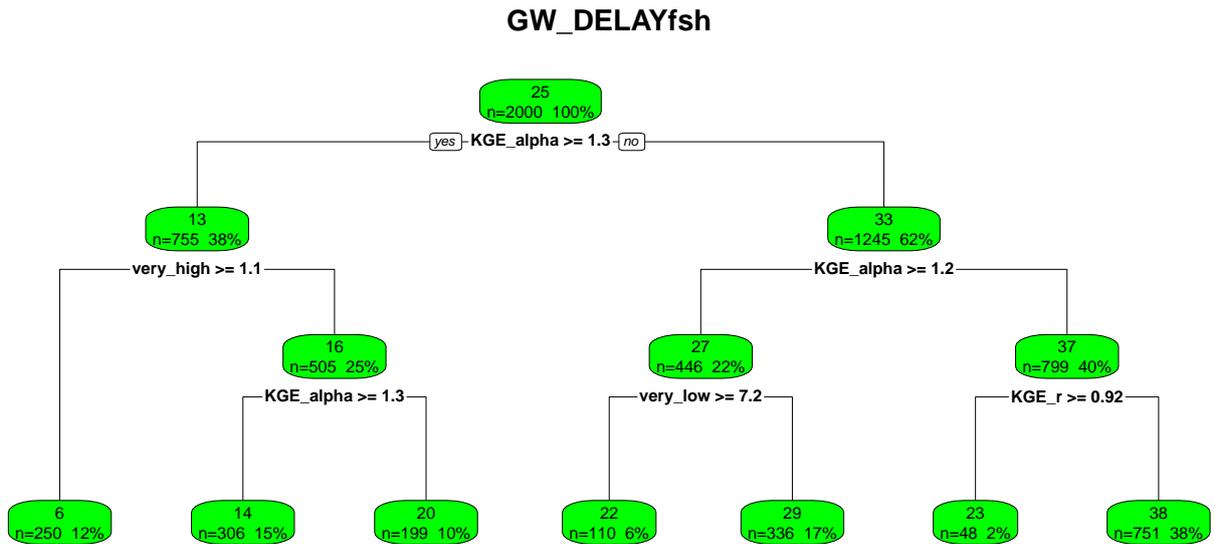
**Figure 4.** Example of a regression tree (RT) using (above) KGE as target variable and model parameters as explaining variables and (below) the model parameter GW\_DELAYfsh as target variable and performance measures as explaining variables for the Treene catchment.
