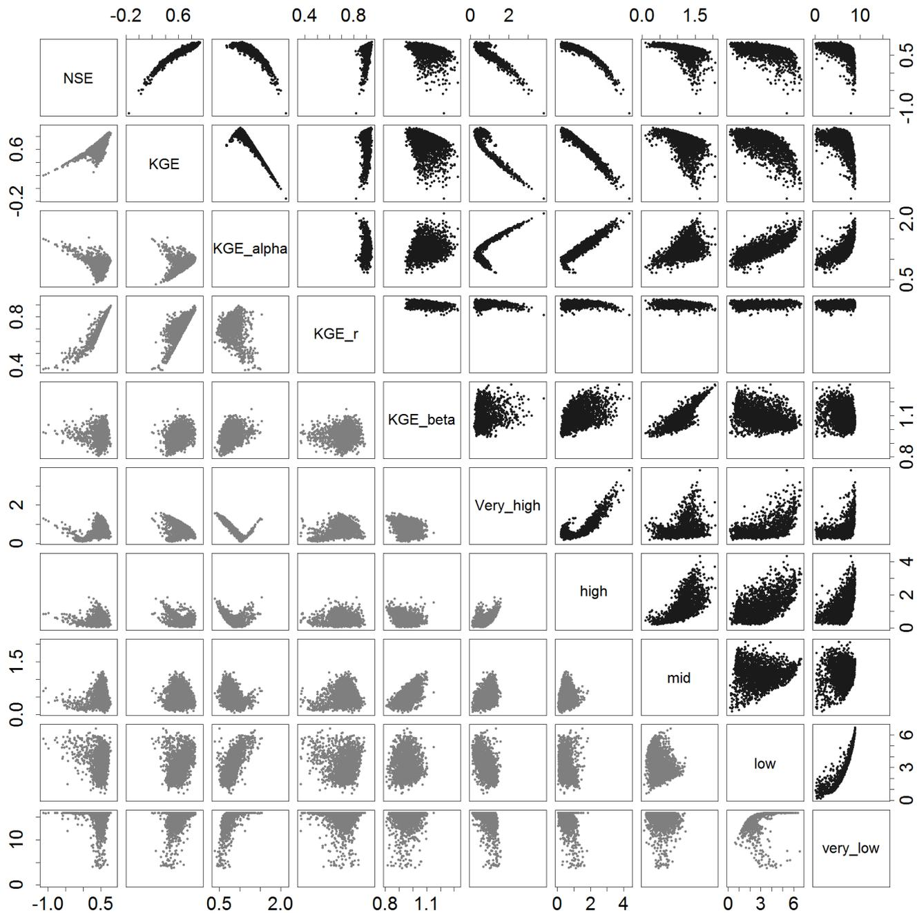
**Figure 3.** Scatterplot matrix of performance criteria of Treene (in black, upper panel) and Saale (in grey, lower panel) catchment showing pairwise performance criteria plots for 2000 model simulations. The scales on the sides show values of the respective performance criterion.
