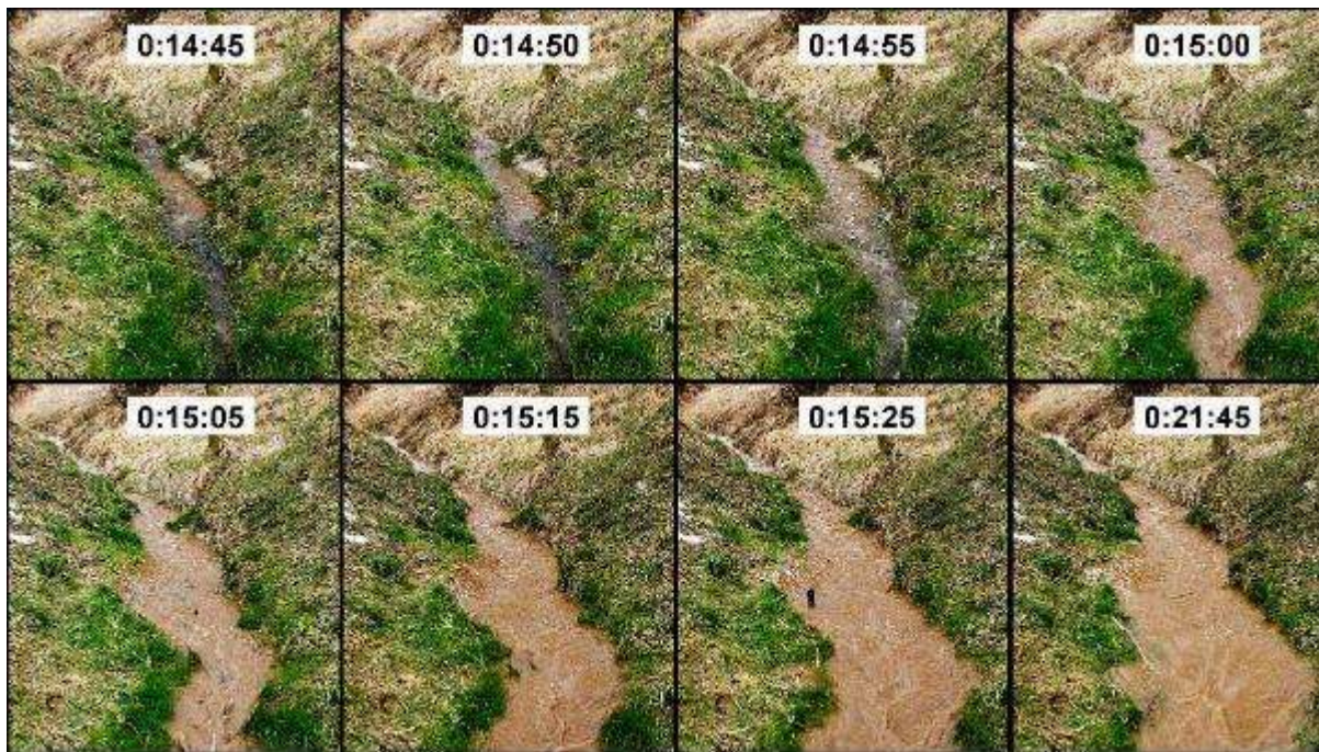
5 Figure 7: The approach of the W4 wave front at stationing of 400 m. The times (h:mm:ss) stand for the duration from the start of the experiment.
