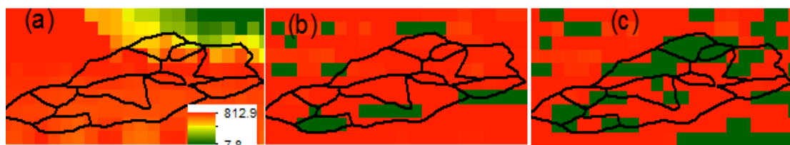
Figure 4 Saturated hydrologic conductivity (mm/day) as derived from (a) large-scale FAO soil dataset, (b) permafrost map of Rieger et al. [1972], and (c) aspect map of CPRW. Panels (b) and (c) are small-scale parameterizations obtained from altering large-scale values according to the presence or absence of permafrost. Grid cells that are classified as permafrost soil are assigned hydraulic conductivity two-orders of magnitude less than the value obtained from the large-scale (FAO) dataset.
