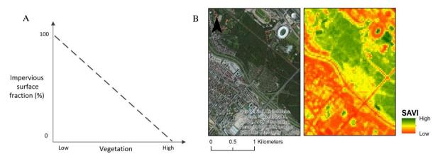
Figure 2: (a) Conceptual relationship between impervious surface fractions and vegetation cover/vegetation indices in urban environments (adapted from Bauer et al., 2008); (b) example of high resolution image, used to measure impervious surface fractions and Soil Adjusted Vegetation Index (SAVI) calculated from Landsat OLI for a central part of Vienna.
