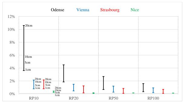
Figure 8: Relative change in flooded area per 1% increase in imperviousness. Results are shown as the range of change for water depths of 1, 5, 10 and 20 cm.
