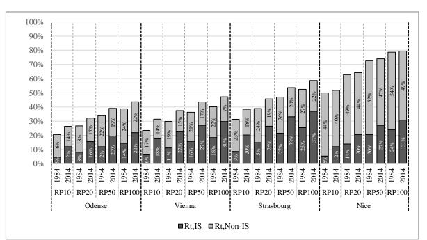
Figure 4: Run-off ratios from urban areas for precipitation events of different intensities, RP10-RP100, divided into shares from impervious (R<sub>t,IS</sub>) and pervious surfaces (R<sub>t,Non-IS</sub>). Run-off ratios are shown for historical (1984) present-day imperviousness (2014 – drainage system as in 1984) and using present-day precipitation intensities.
