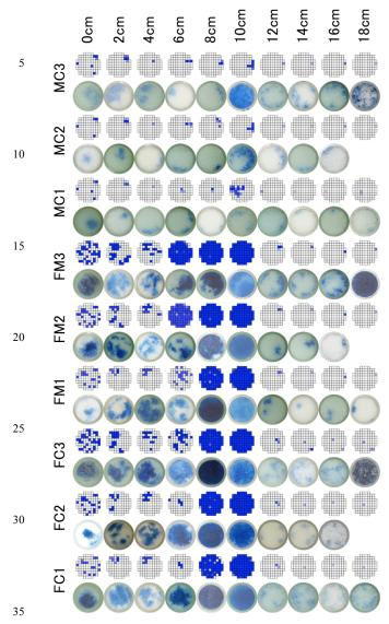
Figure 3: Liquid water distribution (blue shading) at the end of each experiment and simulation. The coordinate on the right denotes the depth of the section from the top surface.
