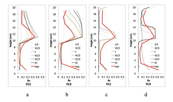
Figure 6: Temporal evolution of simulated water content profiles: (a) FC1 in SNOWPACK, (b) FC3 in SNOWPACK, (c) FC1 in 5 3D model, and (d) FC3 in 3D model. Six profiles are shown in units of the measured arrival time (t).
