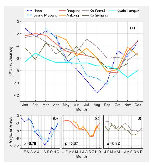
Figure 8: Seasonal monthly mean  $\delta^{18}$ O values for An Long and GNIP data from the Indochinese Peninsula. The data is grouped according to similar variability tested with the Levene test. The p-values given in (b) to (d) are the test statistics. High values indicate similar variance.
