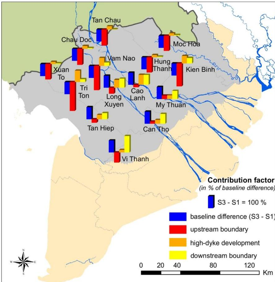
**Figure 10.** Contribution of each factor to the alteration of water levels between the floods 2000 and 2011 for key gauge stations in the VMD. The difference between the two scenarios S3 and S1 is considered to be 100%.
