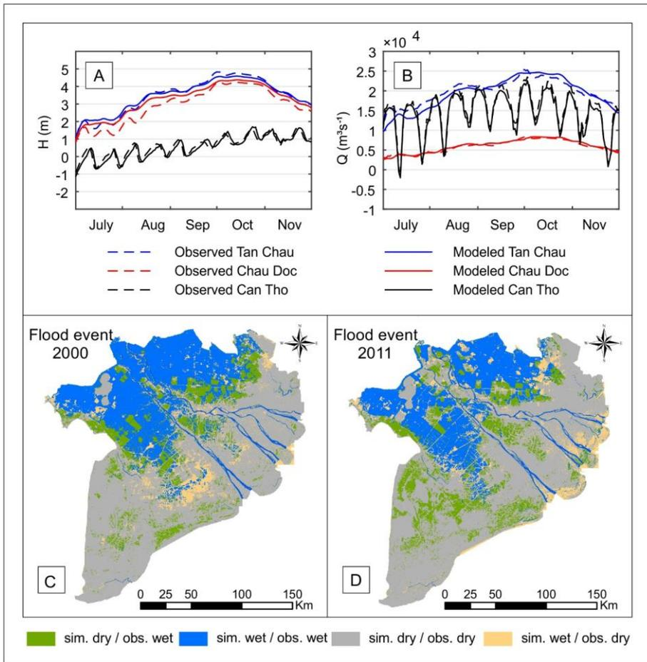
**Figure 4.** Model performance: comparison of gauged and simulated water level (a) and discharge (b) at stations Tan Chau, Chau Doc and Can Tho for the 2011 flood; comparison of observed i.e. derived from satellite data and simulated maximum inundation extent for the floods in 2000 (c) and 2011 (d). Grey and blue color indicate agreement, green color means observed inundation but no inundation simulated, and yellow implies simulated inundation but no inundation observed.
