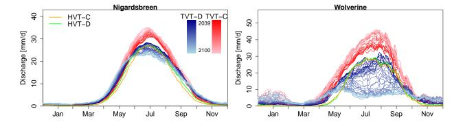
Figure 6 pught thresholds for the four different scenarios HVT-C, HVT-D, TVT-C and TVT-D. The colour gradient for both transient thresholds (blue and red) indicates the adaptation of the threshold each year (for 2039-2100). The thresholds are shown for the Nigardsbreen (left) and Wolverine (right) catchments for climate scenario RCP 4.5.
