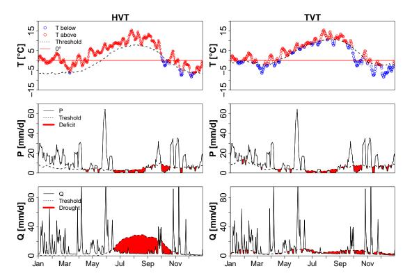
**Figure 9.** Example of streamflow drought and causing factors (T and P) for the different threshold methods. Temperature, precipitation and discharge time series are presented for the Wolverine catchment for 2091, based on climate scenario RCP 4.5 and the dynamical glacier area conceptualisation. For the P and T time series a 7-day moving average was used.
