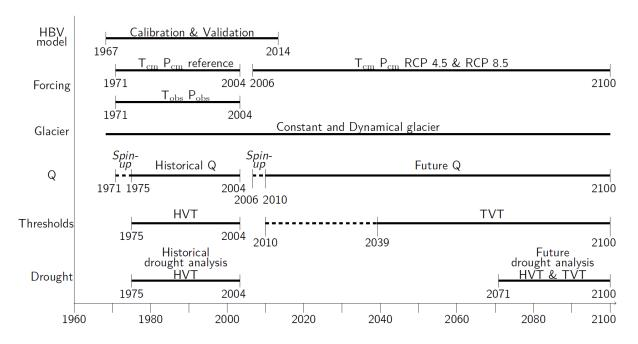
re 2. Timeline indicating the simulation periods, forcings and periods for threshold derivation and application. The different glacier area conceptualisations, constant and dynamical, are used in all simulation periods.
