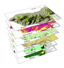
Fig. 2. Figure 2. Geotechnical and environmental factors that affect triggering of landslides on western Hong Kong Island.
