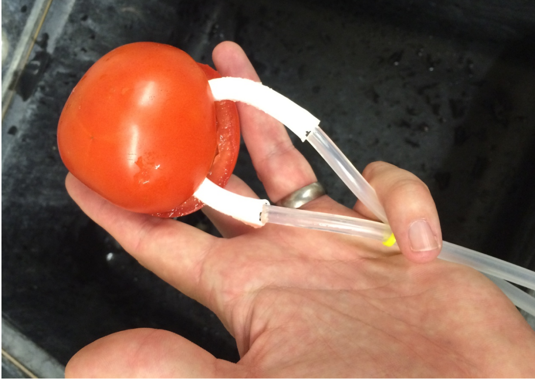
Figure 2. Photograph of membrane-inlet probe (opaque white tubing) partially inserted into a tomato.
