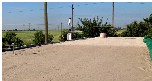
Figure 2. The view over ASSESS from 0 – 19 m shows the tensiometer, the weatherstation, and the groundwater well (left to right) as well as the color of the different sand types (figure adapted from Jaumann (2012)).
