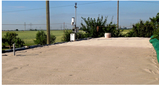
Figure 1. View of ASSESS site with tensiometer access tube, weatherstation, and groundwater well along the left boundary. The jump in color reveals different sands that crop out at the surface (figure adapted from Jaumann (2012)).
