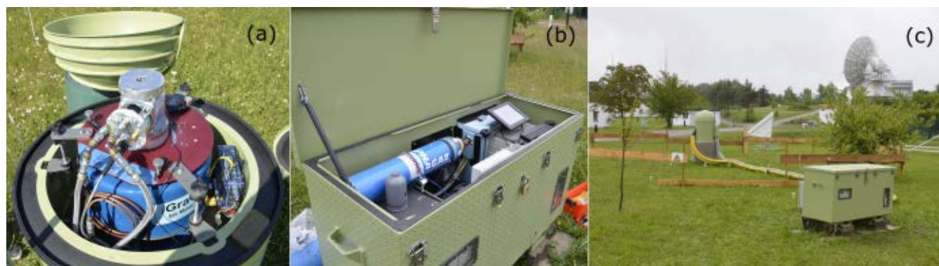
Figure 2: Photographs of the gravimeter monitoring system with (a) the iGrav inside the iGFE field enclosure, (b) peripheral hardware inside the iBox, and (c) an overall view of iBox (foreground), dome-shaped iGFE, and the yellow connection hoses. Photos taken on a grassland site of the Geodetic Observatory in Wettzell, Germany.
