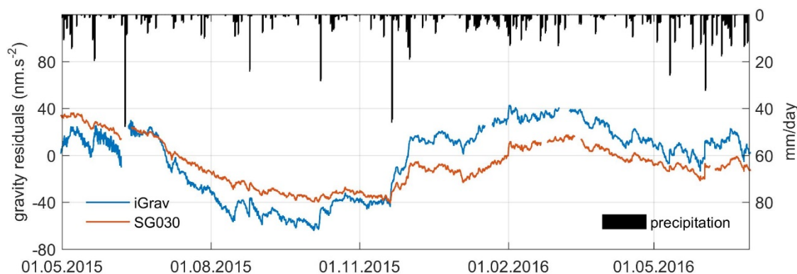
Figure 3: Time series of gravity residuals of iGrav006 in the field enclosure and of SG030 in the observatory building, and daily precipitation rates (from top and right axis) at the Observatory Wettzell.
