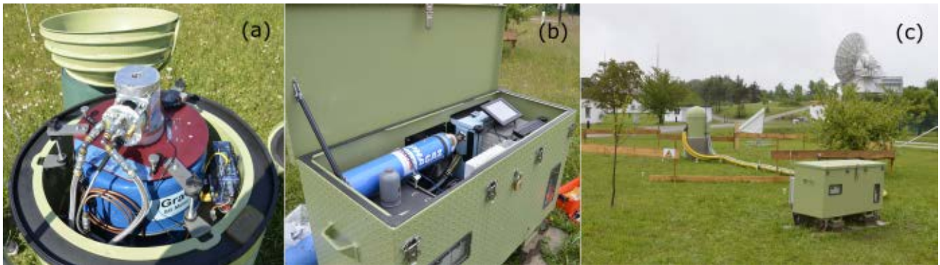
25 Figure 2: Photographs of the gravimeter monitoring system with (a) the iGrav inside the iGFE field enclosure, (b) peripheral hardware inside the iBox, and (c) an overall view of iBox (foreground), dome-shaped iGFE, and the yellow connection hoses. Photos taken on a grassland site of the Geodetic Observatory in Wettzell, Germany.
