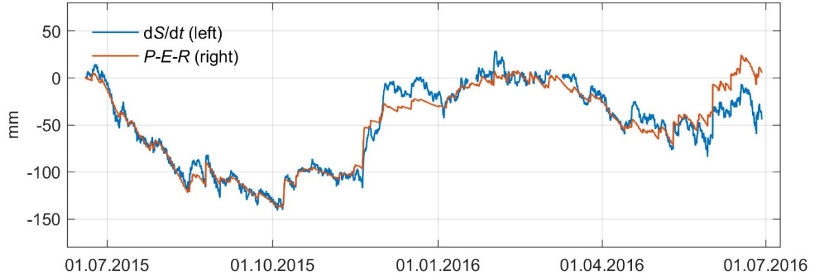
Figure 10: Time series of water storage at Wettzell (as a deviation from the initial storage value at the beginning of the study period, arbitrarily set to 0), with the measured iGrav006 gravity-based storage time series (blue line) (left side of Eq. (3)) and the optimized storage time series (red line) after optimization following the right side of the water balance equation (Eq. (3)).
