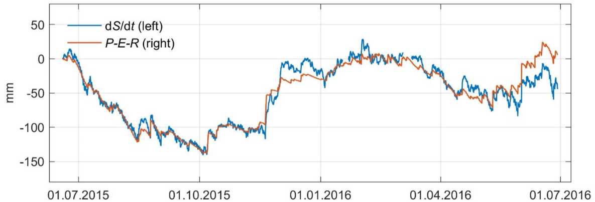
Figure 10: Time series of water storage at Wettzell (as a deviation from the initial storage value at the beginning of the study period, arbitrarily set to 0), with the measured after optimization with iGrav006 gravity-based storage time series on the left (blue line) (left side of Eq. (3)) and the optimized storage time series right side (red line) after optimization following the right side of the water balance equation (Eq. (3)).
