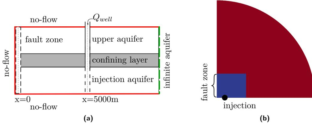
**Figure 5.7.:** a) Cross-section of the domain showing the lateral and top boundary conditions as well as the injection well and the fault zone (modified after ?).
