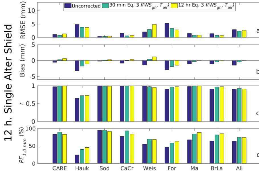
Figure A2. Error statistics for 12 h single-Alter shielded precipitation measurements that are uncorrected (blue), corrected using the 30-min derived transfer functions (green), and corrected using the 12 h derived transfer functions (yellow) are compared.
