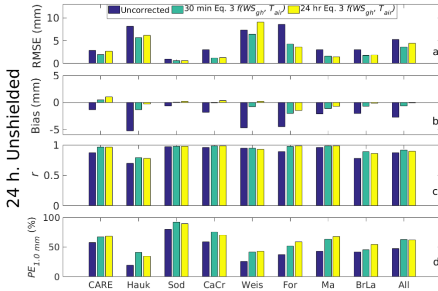
5 Figure A3. Error statistics for 24 h unshielded precipitation measurements that are uncorrected (blue), corrected using the 30-min derived transfer functions (green), and corrected using the 12 h derived transfer functions (yellow) are compared.
