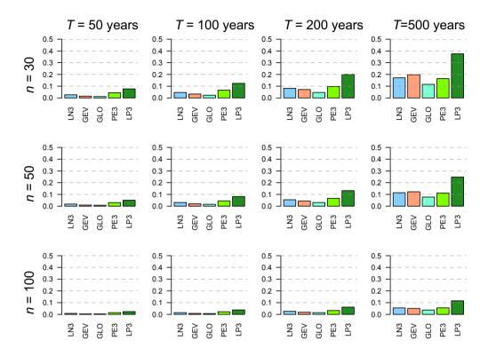
Figure 3. Values of the correction factor  $\hat{y}$  from Eq. (6) for some values of the sample length n and return period T and for different three-parameter fitting distributions (LN3 = log-Normal; GEV= generalized extreme value; GLO = generalized logistic; PE3 = Pearson type III; LP3 = log Pearson type III). The LP3 corresponds to the PE3 with log-transformed variate.
