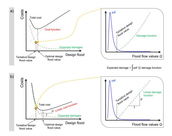
**Figure 1.** Illustrative example (without uncertainty) of the application of the cost-benefit framework to compute the design flood. Two generic cost and damage functions are reported in panel a, while panel b shows the linear functions adopted in the UNCODE framework.
