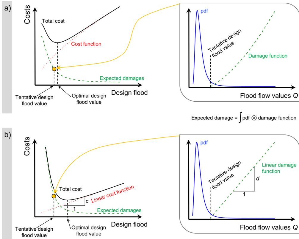
**Figure 1.** Illustrative example (without uncertainty) of the application of the cost-benefit framework to compute the design flood. Two generic cost and damage functions are reported in panel a, while panel b shows the linear functions adopted in the UNCODE framework.
