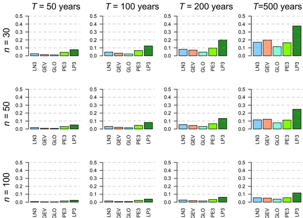
**Figure 3.** Values of the correction factor  $\hat{\gamma}$  from Eq. (6) for some values of the sample length  $n$  and return period  $T$  and for different three-parameter fitting distributions (LN3 = log-Normal; GEV= generalized extreme value; GLO = generalized logistic; PE3 = Pearson type III; LP3 = log Pearson type III). The LP3 corresponds to the PE3 with log-transformed variate.
