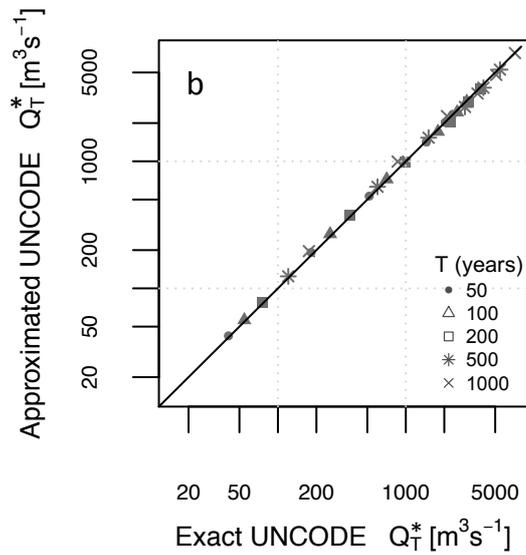
**Figure 2.** Comparison between the exact,  $Q_T^*$ , and the approximated,  $\hat{Q}_T^*$ , UNCODE estimators of the design flood for a pool of 6 flood records considered in Botto et al. (2014, Table 1) with at least 30 years of data. Different return periods are listed in the legend. The reference distribution used for this flood frequency analysis is the 3-parameter log-Normal (LN3) in panel “a” and the generalized extreme value (GEV) in panel “b”.
