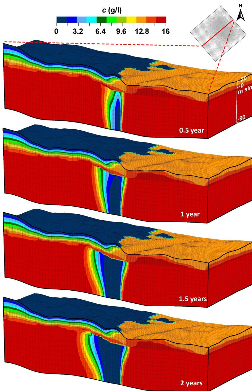
15 Figure 14. Scenario  $S_{3A}$ : evolution of the salt concentration (g/l) on a vertical section through the barycenter of the injection configuration. Vertical exaggeration is 10.
