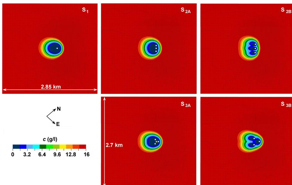
10 Figure 13. Salt concentration (g/l) on a horizontal plane at -30 m amsl (i.e., at the top of the injected aquifer) after 2 years of aquifer recharge for the various scenarios addressed by the study. The location of the injection wells are shown by white dots. The production well in scenario S<sub>3A</sub> is marked by a yellow X mark.
