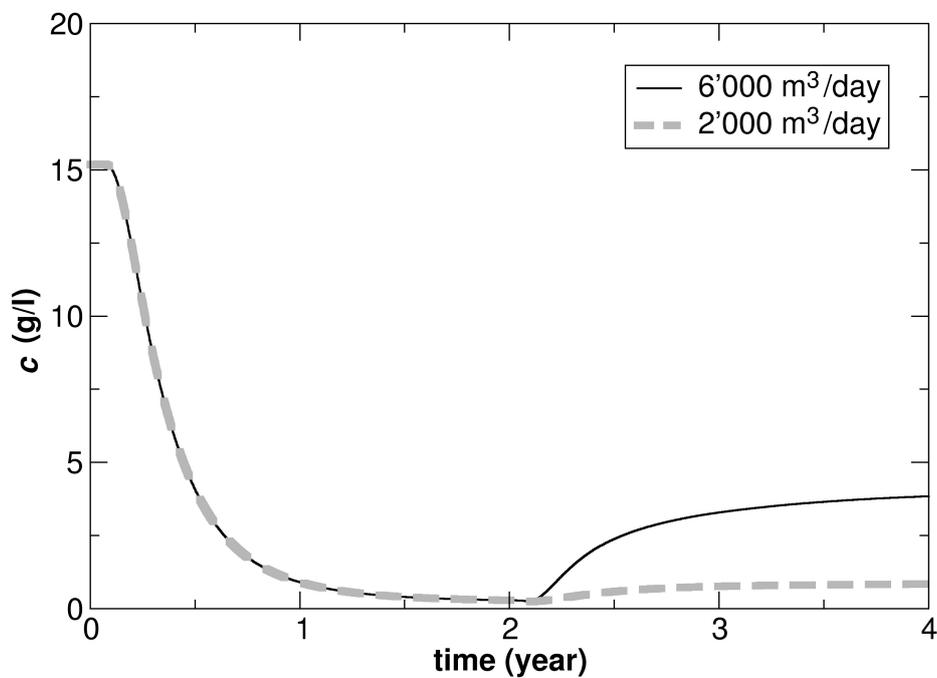
Figure 15. Salt concentration versus time at the pumping well intake for the two selected values of  $Q_{\text{withdrawn}}$ .
