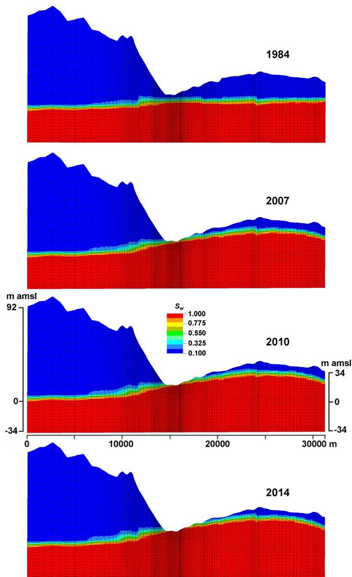
Figure 9. Evolution of the saturation degree along the vertical cross-section E-E traced in Figure 2, i.e. along the main groundwater flow direction, as obtained by the 3D depression-scale model.
