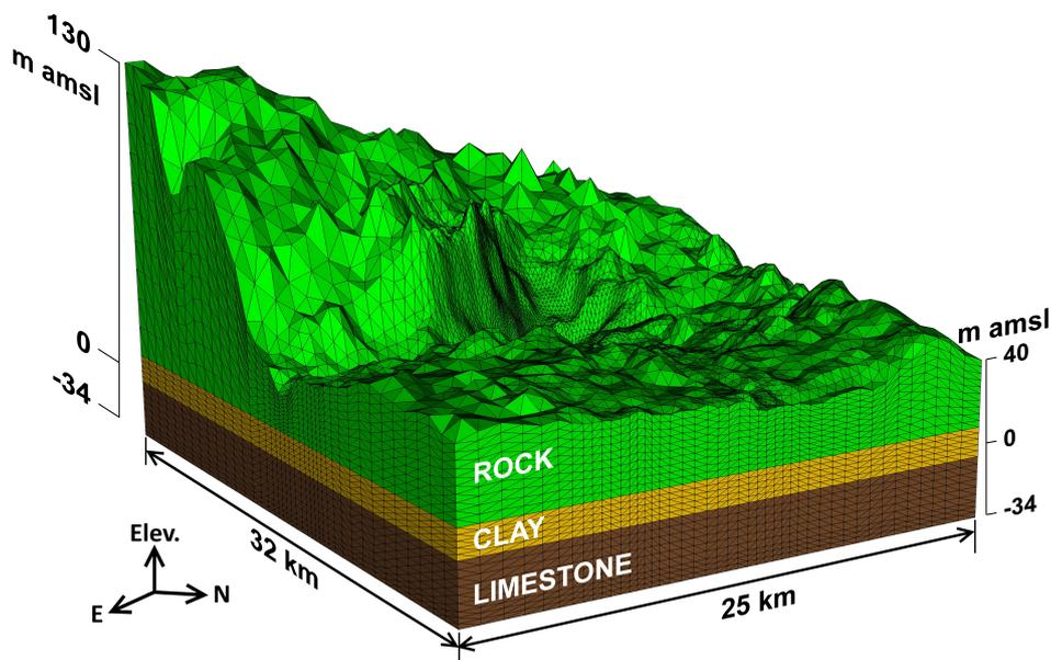
90 Figure 8. 3D mesh of the regional hydrogeological model. A 2D triangular grid was projected vertically to generate the 3D FE tetrahedral mesh used in the CATHY simulations.
