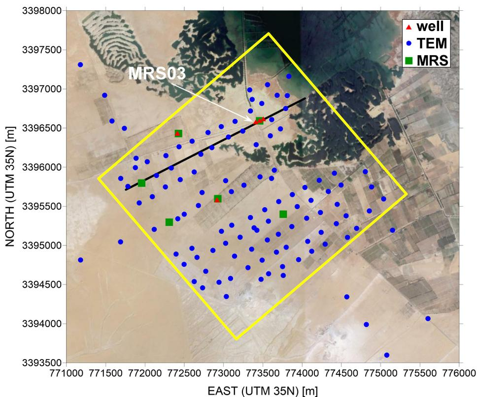
70 **Figure 5.** Location map of the boreholes (red triangles), TEM (blue dots) and MRS (green squares) measurements carried out in the surroundings of the Nubariya pond. The black line represents the trace of the cross section through the resistivity model shown in Figure 6. The location of MRS03 is highlighted. The domain of the local-scale model is shown by the yellow box. The background is a Landsat image acquired in 2014.
