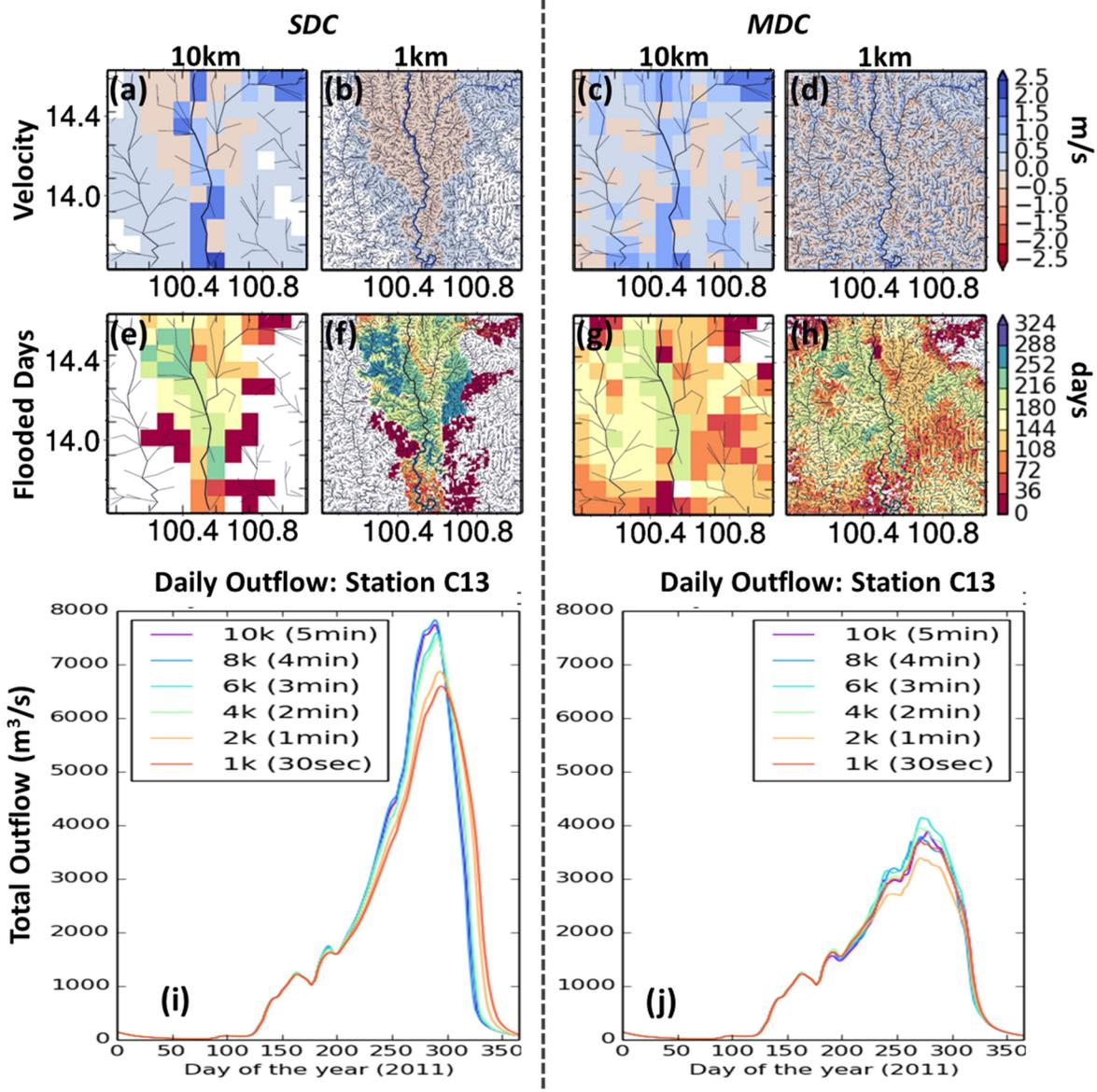
Figure 8. Impacts of spatial resolution and representation of *MDC* to (a – d) flow velocity, (e – h) number of days of flooding in a year, and (i – j) 2011 daily outflows (river + floodplain flows) at C13 Station. Figures a to h show simulation results at the lower part of the basin.
