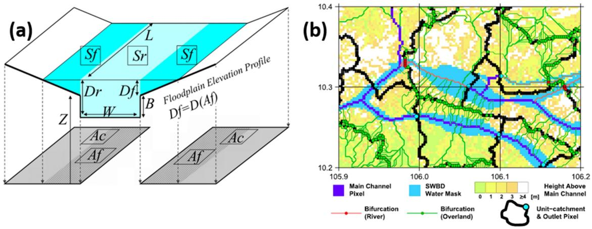
**Figure 2. Schematic diagram of CaMa-Flood.** (a) River channel and floodplain sub-grid parameters (modified from Yamazaki et al., 2011). Please refer to Table 1 for definition of variables. (b) Sub-grid topography and MDC channels. Overland pathways are represented by the green channels while river pathways are represented by the red channels (modified from Yamazaki et al., 2014b).
