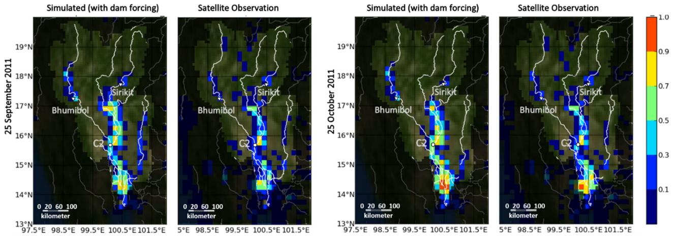
5 **Figure 3. Validation of SDC simulation at 10k resolution.** The simulated (a) daily discharge for the years 2010-2011 and the (b) monthly discharge from 1981-2004 were compared with the naturalized observed discharge. The (c) ratio of inundated area in September 25, 2011 and October 25, 2011 were compared with satellite data. Dam forcing indicates the simulations constrained using actual dam outflows as boundary conditions. All figures were modified from Mateo et al. (2014).
