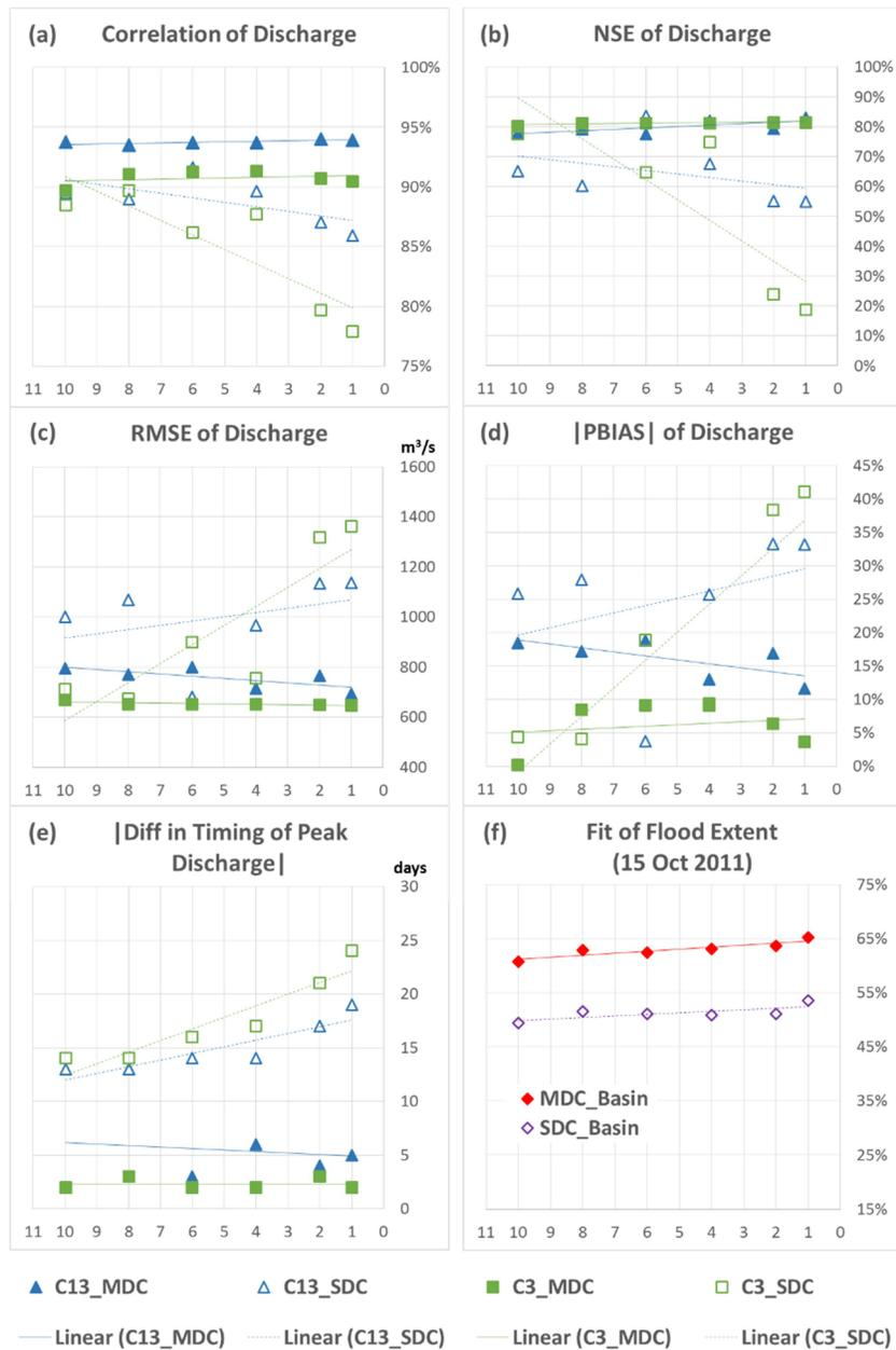
5 **Figure 5. Model efficiency at varying spatial resolution and varying flow connectivity schemes.** The statistics for discharge (Correlation, RMSE, Percent Bias, NSE Coefficient, and difference in peak timing) were calculated and compared with the naturalized discharge at corresponding gauge stations. The fit of flood extent was calculated for the entire basin.
