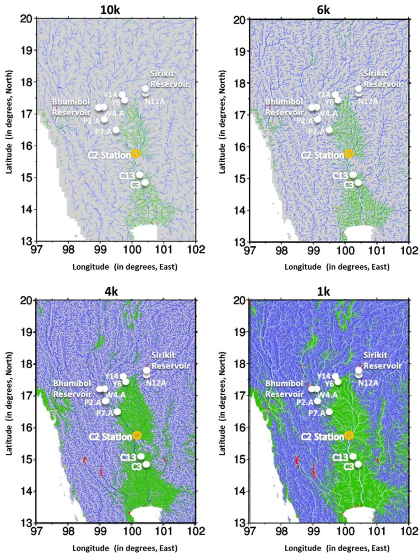
**Figure 4. Change in the density of MDC pathways with spatial resolution.** The density of river network and MDC pathways increase with increasing spatial resolution. Gauge stations upstream of C2 Station (Y14, Y6, N12A, W4A, P2A, and P7A) are located in zones with low density of MDC pathways. Gauge stations C2, C13, and C3 are located in low-lying and floodplain areas which have a high density of
