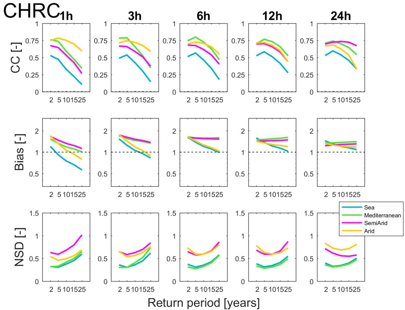
**Figure 8: Comparison of IDF values between CHRC and radar for different climatic regions. Blue lines represent sea areas while green, pink and orange lines represent Mediterranean, semiarid and arid climates respectively. The first row of panels shows the CC for different durations, the second row the Bias and the third row the NSD.**
