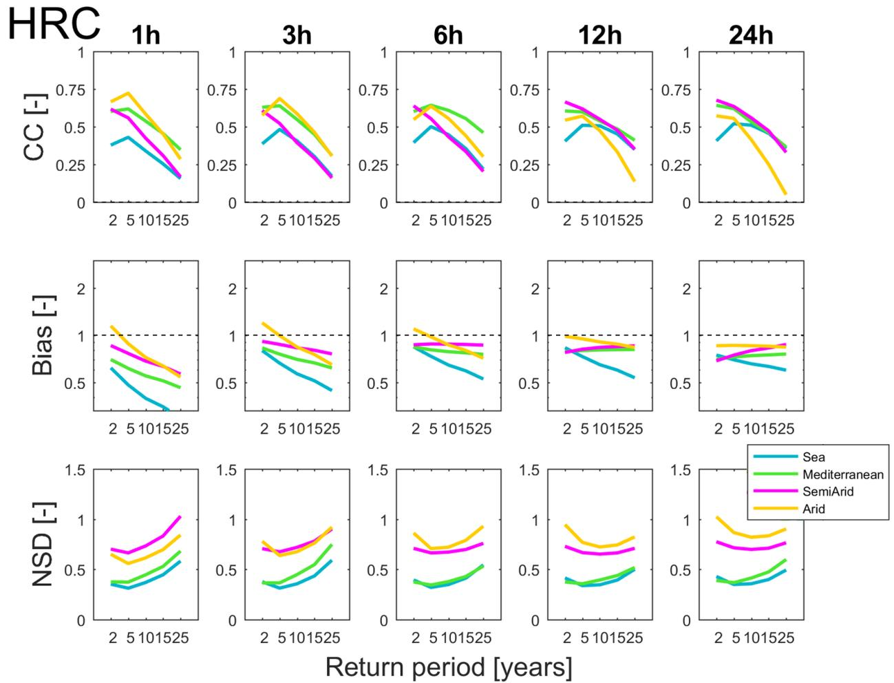
5 **Figure 7: Comparison of IDF values between HRC and radar for different climatic regions. Blue lines represent sea areas while green, pink and orange lines represent Mediterranean, semiarid and arid climates respectively. The first row of panels shows the CC for different durations, the second row the Bias and the third row the NSD.**
