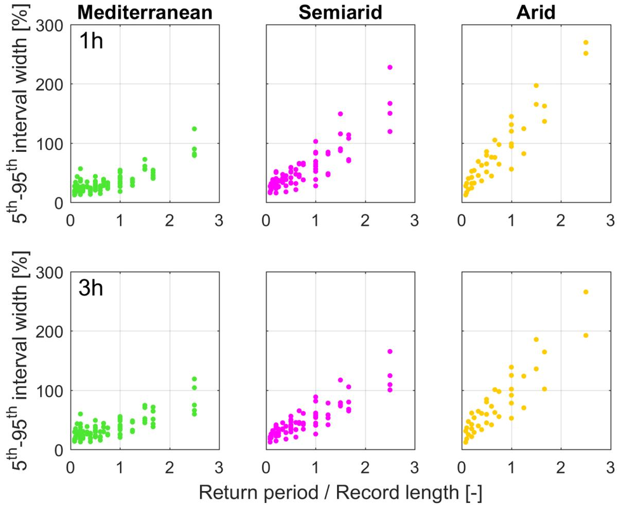
**Figure 10:** Relative uncertainty (width of the 5-95<sup>th</sup> quantile interval of the 999 bootstrap sampling repetitions normalized over the rain gauge-IDF value) plotted against the ratio between the estimated return period and the record length. The first row of panels shows the results for 1 h duration, the second row for 3 h. Columns of panels show results for each climatic region.
