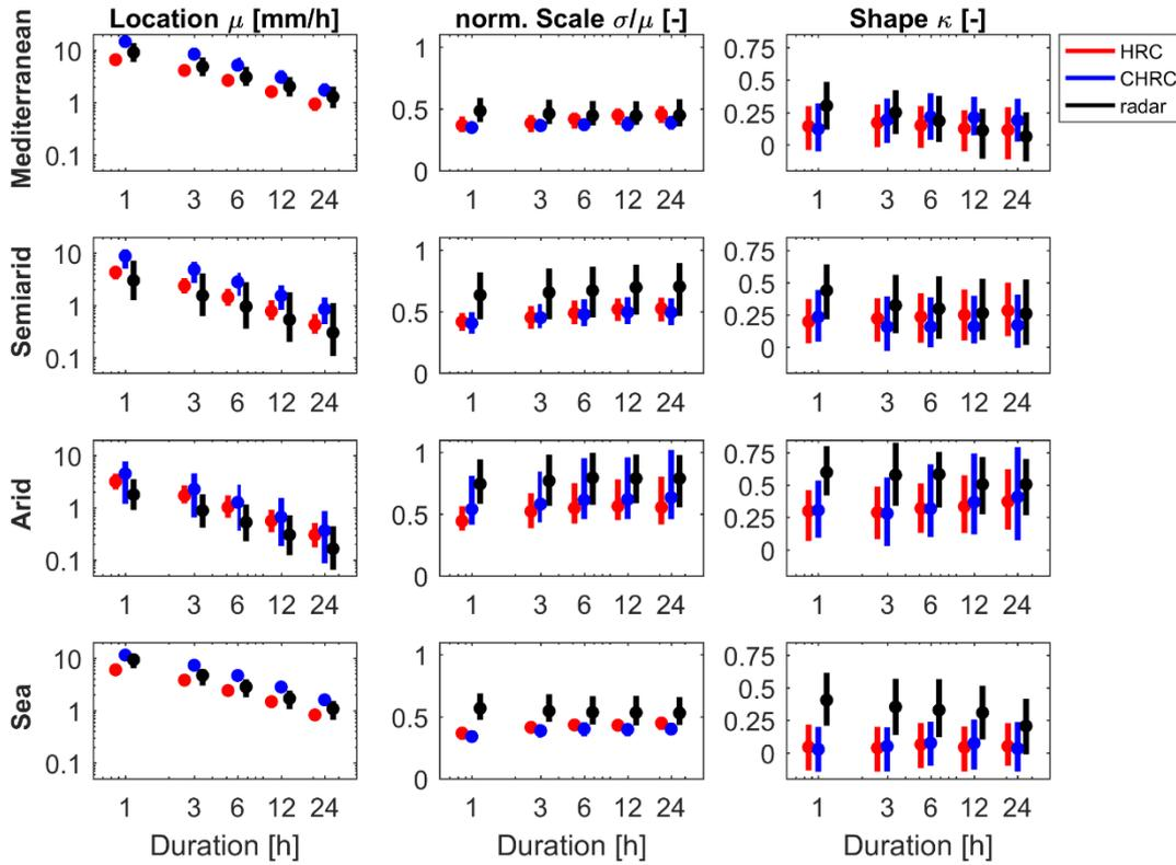
Figure 2: Distribution (median and 25<sup>th</sup>-75<sup>th</sup> quantiles) of the GEV parameters derived from satellite (HRC and CHRC) and radar datasets. Note that scale parameters are normalized over the corresponding location parameters. The parameters for different products are represented around the corresponding duration so the logarithmic scale in x-axes should be interpreted accordingly.
