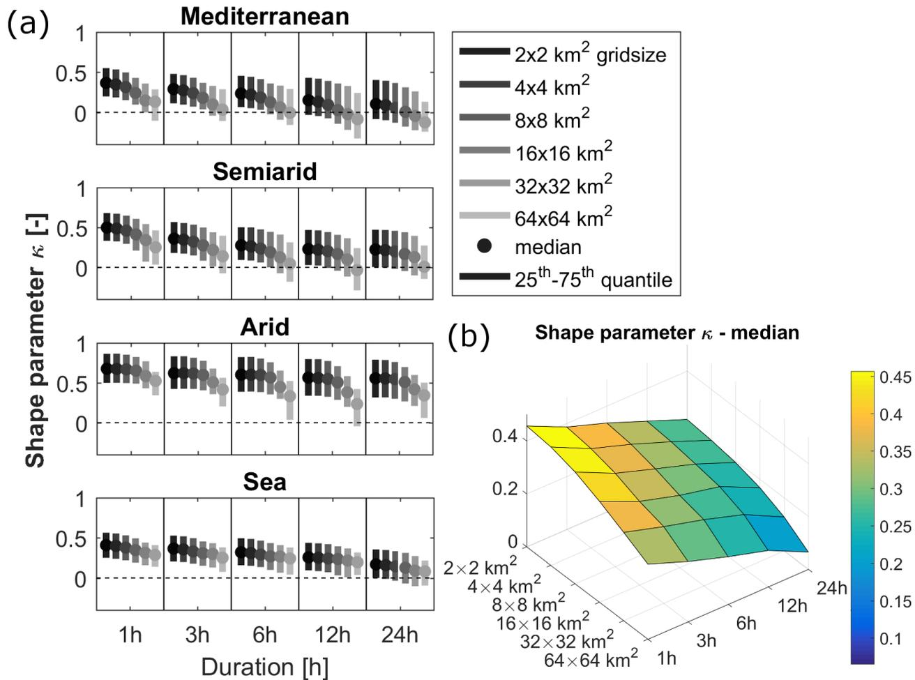
Figure 3: (a) Distribution (median and 25<sup>th</sup> -75<sup>th</sup> quantiles) of the shape parameters derived aggregating radar estimates on grid sizes increasing from 2x2 to 64x64 km<sup>2</sup>. (b) Median of the shape parameters (all climates) derived aggregating radar estimates as a function of the spatial and of the temporal aggregation scales.
