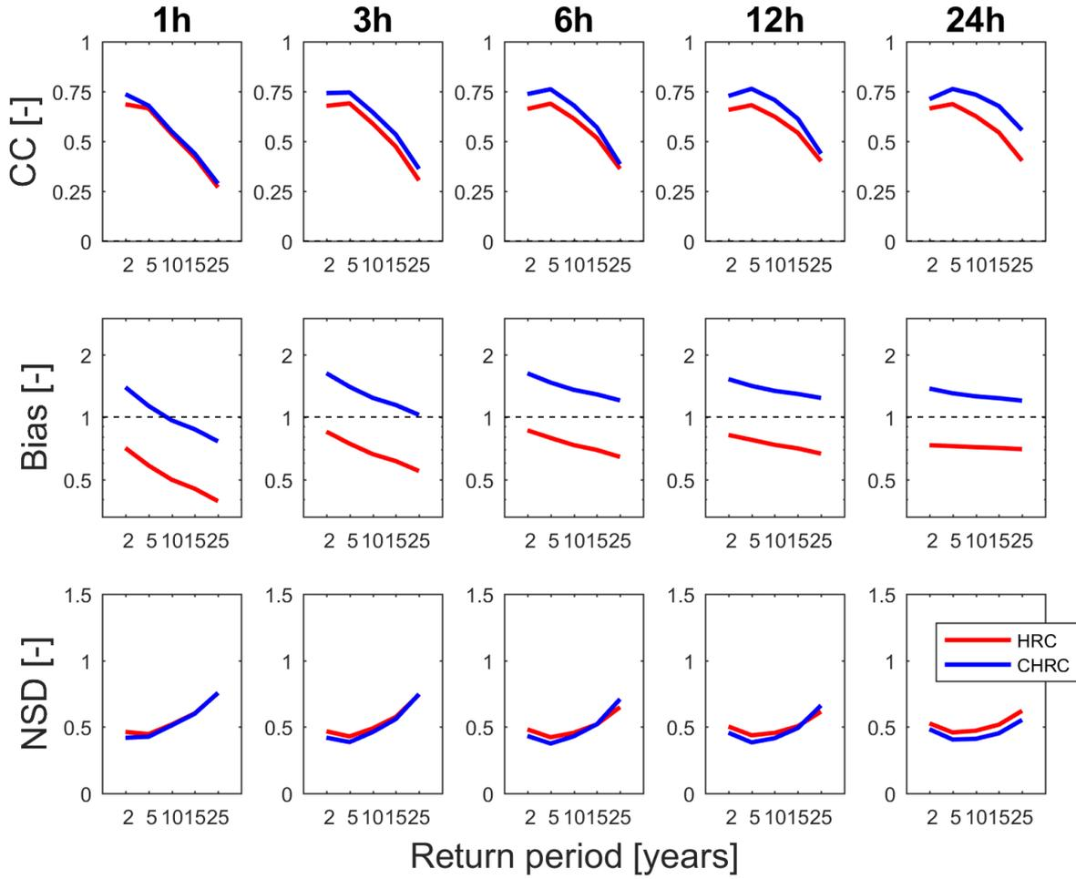
**Figure 6: Comparison of IDF values between HRC and radar (red) and CHRC and radar (blue). The first row of panels shows the CC for different durations, the second row the Bias and the third row the NSD.**
