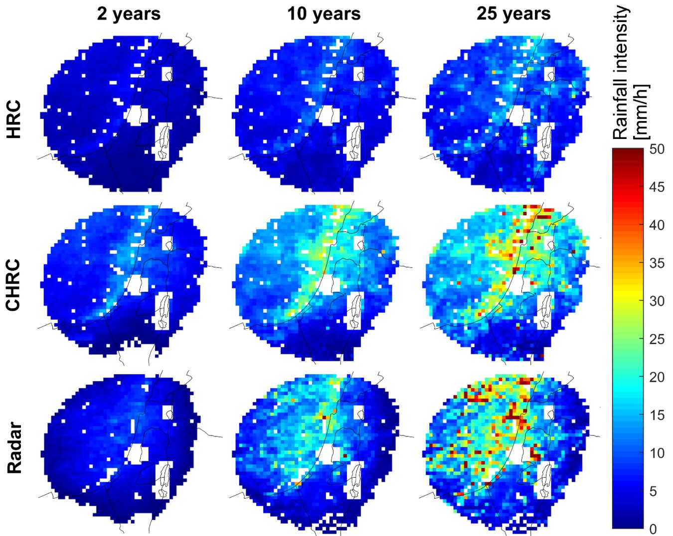
**Figure 5: Example of IDF maps for 3 h duration from HRC, CHRC and radar for 2, 10 and 25 years return periods. Only the pixels included in the analyses are shown.**
