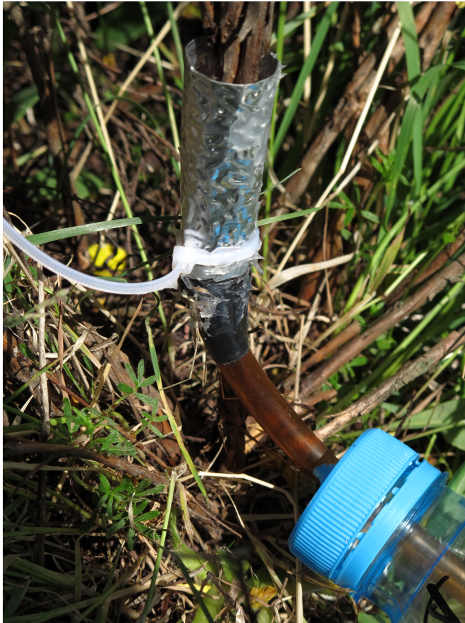
Fig. 7. Stemflow collection apparatus on a branch (photo courtesy of Si-Yi Zhang)
