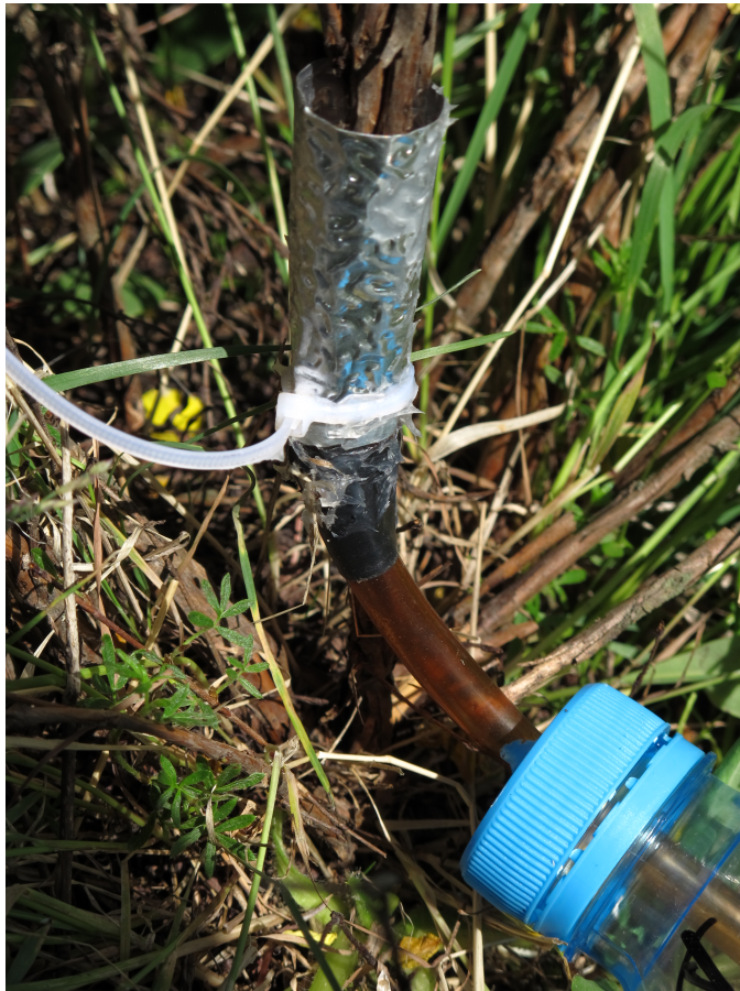
Fig. 1. Figure 1 Stemflow collection apparatus on a branch
