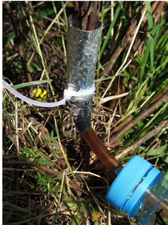
Fig. 1. Figure 1 Stemflow collection apparatus on a branch
