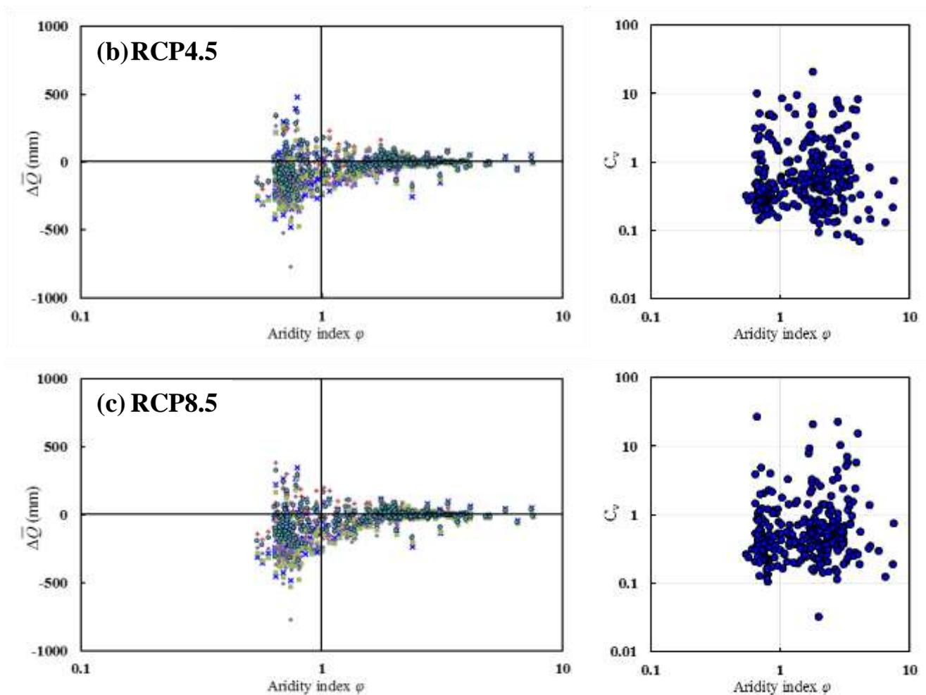
5 **Figure 6: Assessment of the DDWW pattern under (a) RCP2.6, (b) RCP4.5 and (c) RCP8.5 Scenarios. (left)** Relationship between predicted changes in mean annual runoff ( $\Delta\bar{Q}$ ) of five models and the aridity index. **(right)** Coefficient of variance ( $C_v$ ) of predicted runoff changes. Each blue point denotes a catchment.
