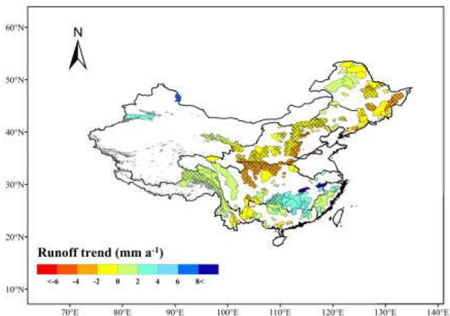
Figure 2: The observed runoff trends in the 291 catchments. Dark red and blue denote catchments with a trend smaller than -6 and larger than 8. Crosshatched areas are significant catchments. Grey shading areas are glaciers based on the second glacier inventory dataset of China (Guo et al., 2014).
