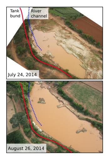
**Figure 2.** Aerial photos of a small tank containing turbid water in the Arkavathy watershed before and after runoff events in August 2014. The tank receives water from the channel and directly from adjacent agricultural plots, and water extent increases with storage.
