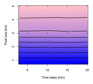
**Figure 4.** Fraction of pixels containing at least one measurement (after filter is applied) for various combinations of time steps and pixel grid size (represented with cross) over the Amsterdam area between December 2014 and April 2016.
