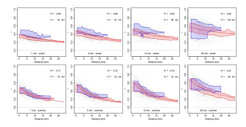
**Figure 11.** Correlograms of all stations after filtering at various accumulation values for winter (top panels) and summer (bottom pannels). The red and blue areas represent the interquartile range of the Netatmo stations and non-Netatmo stations respectively. The areas are constructed with a moving window of width 5 km. The scatter plots are fitted with the exponential relation stated in Eq. (2), which fitting parameters are given in the panels.
