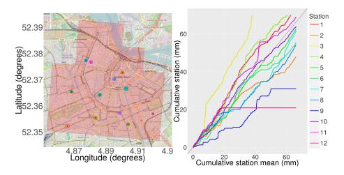
**Figure 9.** Left panel: Locations of 12 stations and 20 radar pixels in the city center of Amsterdam, where symbol size represents the number of unique days with measurements by the station (range 371-514 days). Right panel: Double mass plots of the station measurements as compared to the mean of all 12 stations over the intervals where all stations contain measurements.
