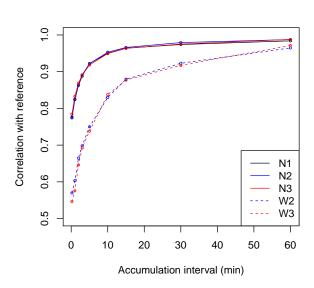
**Figure 6.** Correlation between rainfall measurements by Netatmo stations (N1, N2 and N3), also obtained via Wundermap (W2 and W3), and the pit gauge reference for various accumulation time steps.
