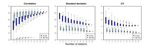
**Figure 10.** Boxplots of correlation, standard deviation and coefficient of variation (CV) of rainfall intensity for all subset means within the 12 stations in Amsterdam city center, as compared to the radar rainfall intensity 20 pixel mean for interpolated 5 minute and hourly time series.
