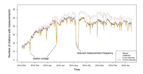
**Figure 3.** Number of stations with rainfall data from the PWS dataset, before and after applying filter, for every 5 and 10 minute interval over the entire period, smoothed per day. The two indicated dips corresponds to complete outage of stations, the third with a longer period of fewer measurements in all stations.
