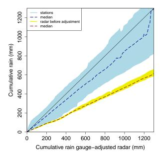
**Figure 7.** Double mass plots of station filtered rainfall measurements and real-time available radar data with gauge-adjusted radar rainfall at the corresponding location in the period between December 2014 and March 2016. Only intervals where both radar and station contain measurements are taken into account. Colored regions indicate the range between minimum and maximum of the graphs and dashed lines represent the median of the combined datasets.
